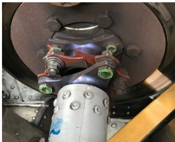
Figure 1. EC135 Tail Rotor flexible coupling failure.
