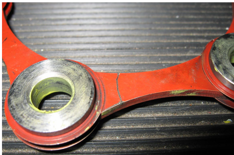
Figure 3. Eurocopter AS365 Dauphin flexible coupling failure.
