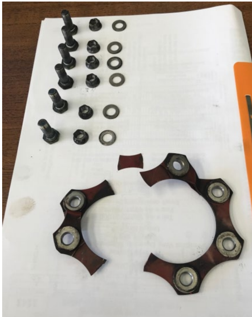
Figure 2. EC135 Tail Rotor flexible coupling failure.
