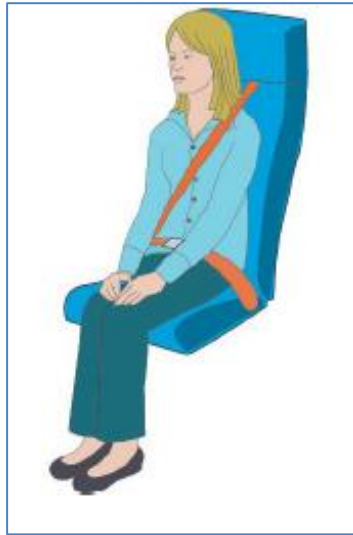
Figure 4: Aft facing passenger seat, with a lap strap and shoulder harness with single diagonal strap
