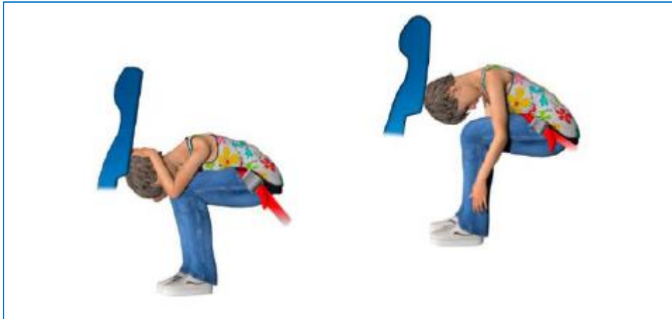
Figure 4: Brace positions in forward facing passenger seats equipped with a lap strap seatbelt only
