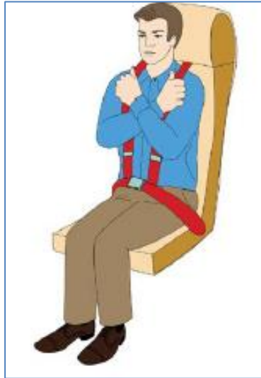
Figure 11: Aft facing seat, lap strap and shoulder harness with dual upper torso straps, onshore helicopter occupant
