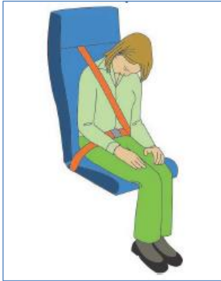
Figure 5: Forward facing passenger seats equipped with a lap strap and shoulder harness with single diagonal strap
