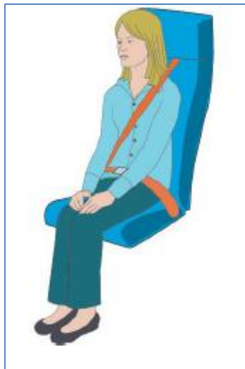
Figure 7: Aft facing passenger seat, with a lap strap and shoulder harness with single diagonal strap (Source: ICAO Doc 10086 Manual on Information and Instructions for Passenger Safety (first edition))
