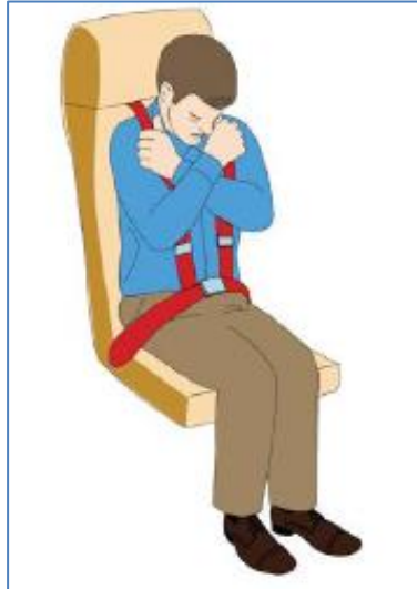
Figure 10: Forward facing seat, lap strap and shoulder harness with dual upper torso straps, onshore helicopter occupant (Source: ICAO Doc 10086 Manual on Information and Instructions for Passenger Safety (first edition))
