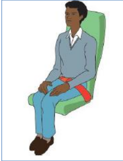
Figure 6: Aft facing passenger seat, with a lap strap only (Source: ICAO Doc 10086 Manual on Information and Instructions for Passenger Safety (first edition))
