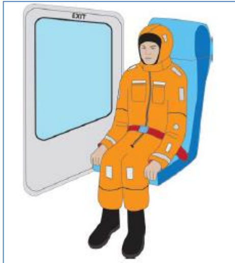
Figure 13: Aft facing seat, lap strap only, offshore helicopter occupant (Source: ICAO Doc 10086 Manual on Information and Instructions for Passenger Safety (first edition))
