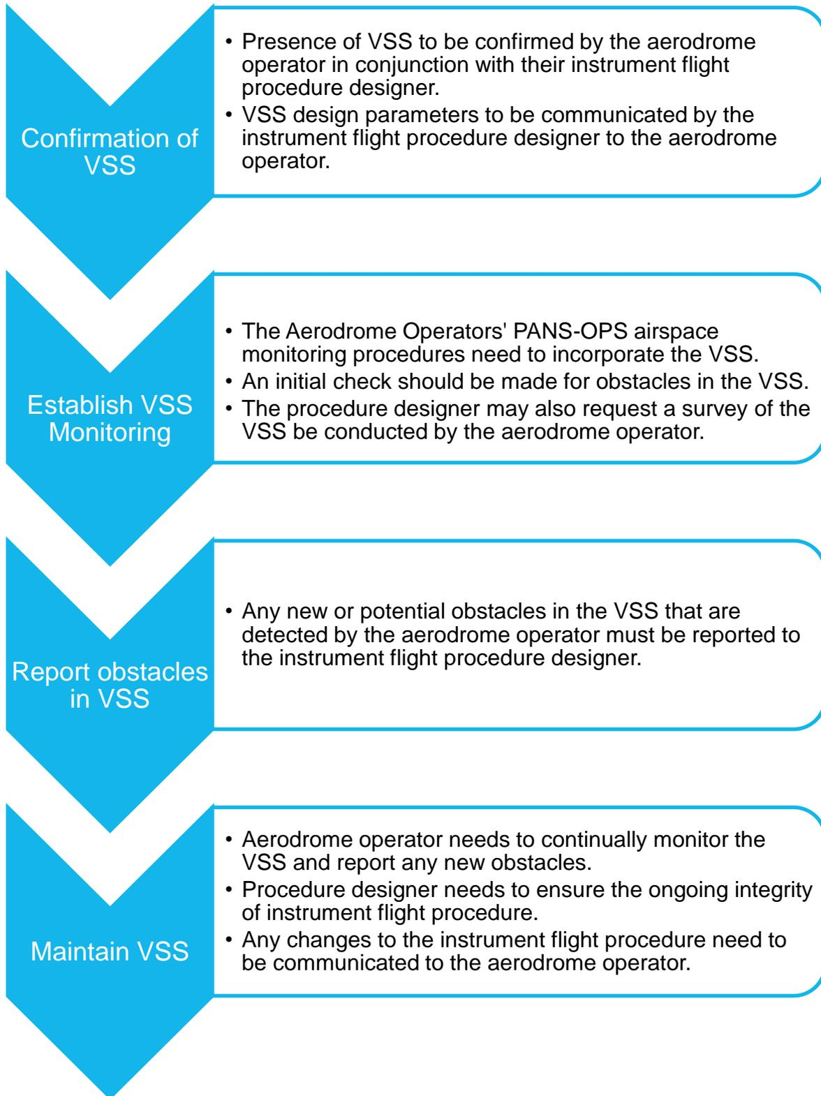
**Figure 1: Recommended approach for VSS obstacle monitoring**
