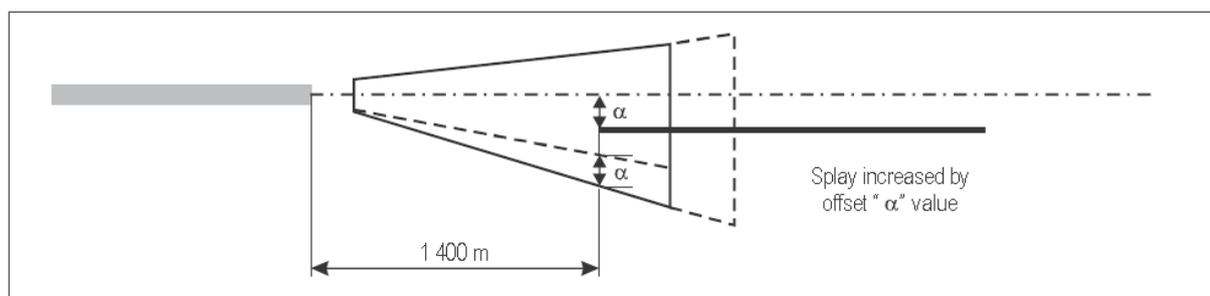
Figure 9: Plan view of VSS with an offset final approach parallel to the runway centre line<sup>7</sup>
