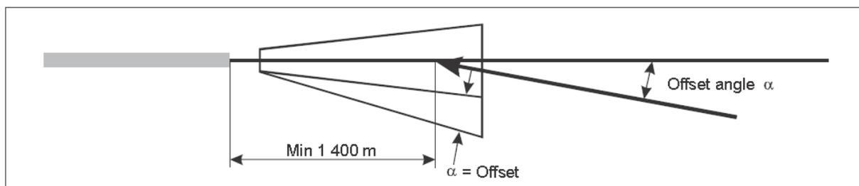
Figure 8: Plan view of VSS for an offset final approach with a runway centre line crossing<sup>6</sup>
