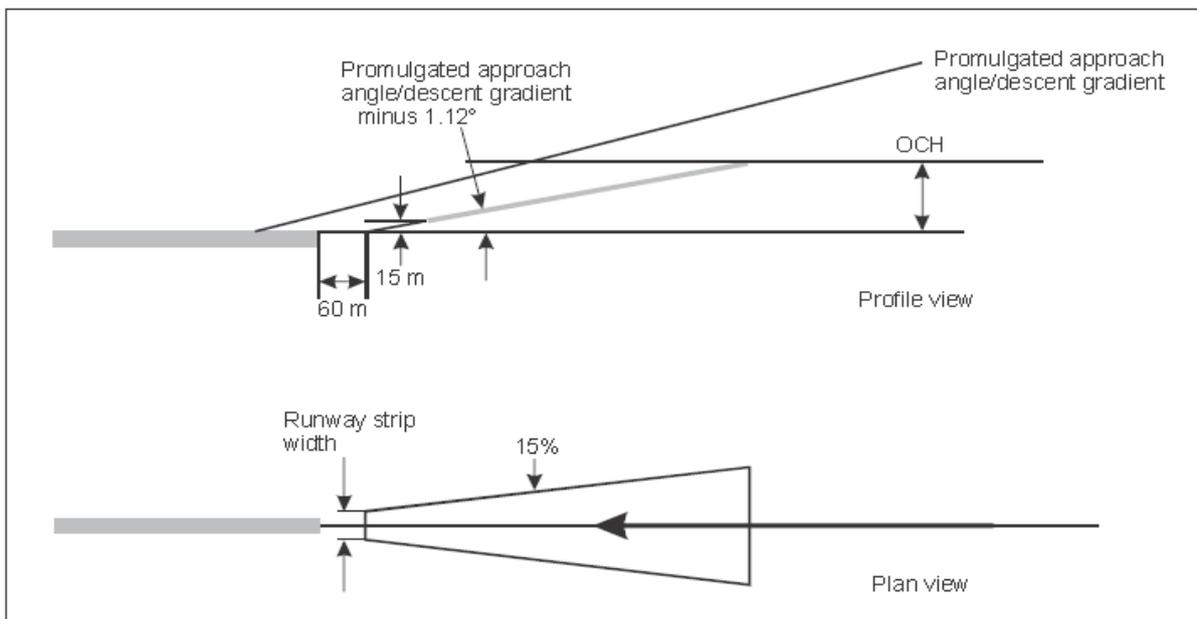
Figure 7: The VSS of other approach procedures for a normal straight-in approach<sup>5</sup>
