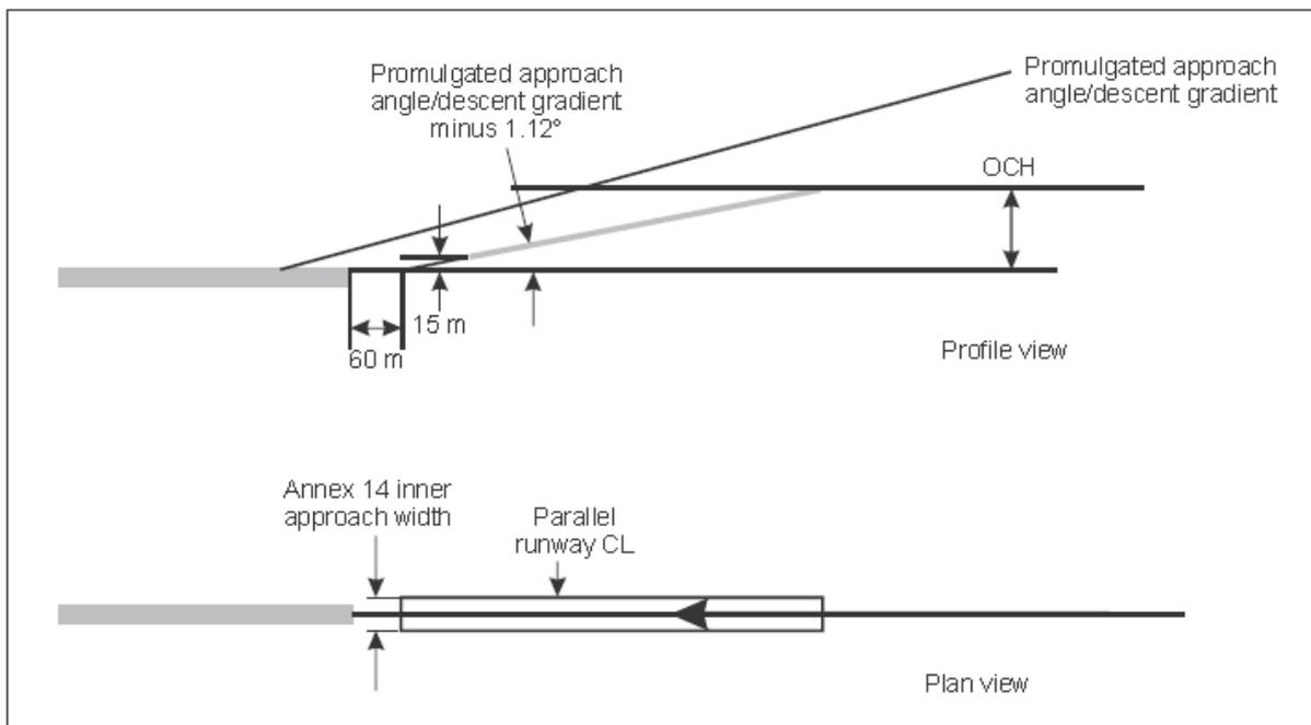
**Figure 6: The VSS of procedures with localizer or localizer look-alike lateral guidance aligned with the runway centreline<sup>4</sup>**
