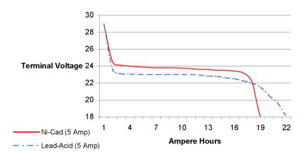
Figure 4: Discharge rates of lead-acid and nickel-cadmium batteries
