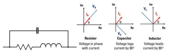
Figure 5: Circuit equivalent components - Impedance
