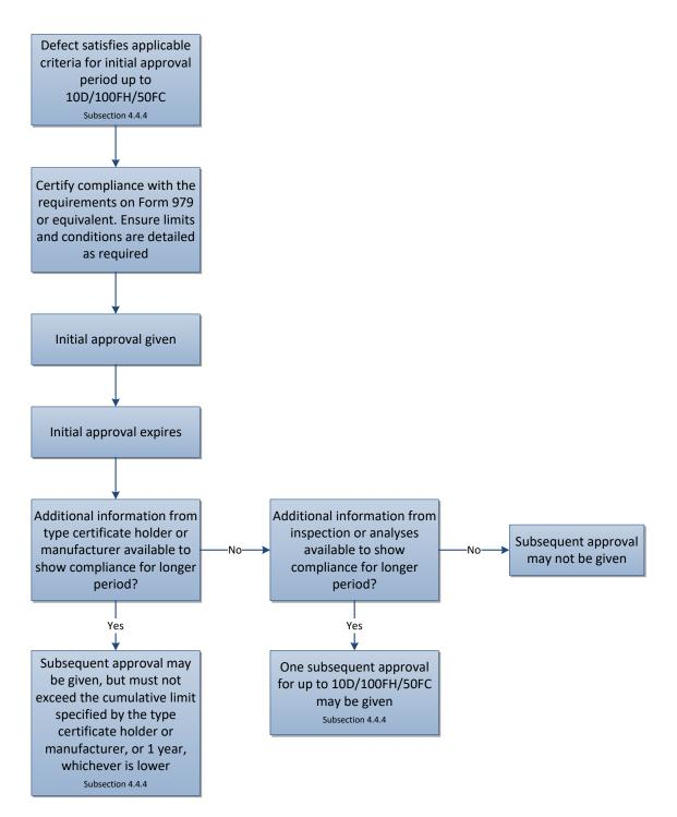
Figure 7: Approval process with 10D/100FH/50FC limit
