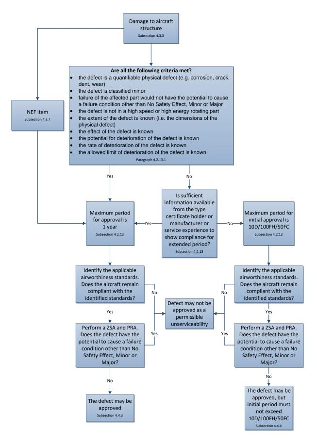
Figure 2: Assessment process for damage to aircraft structure
