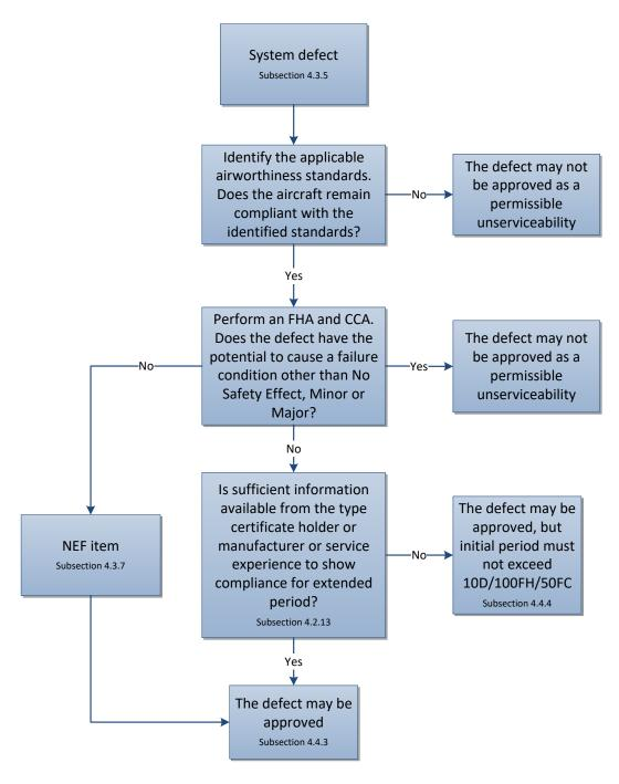
Figure 4: Assessment process for system defects
