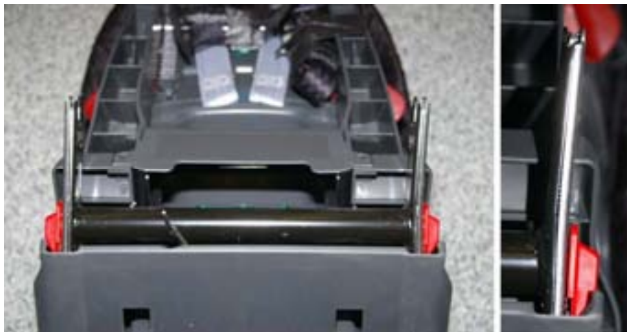
Figure 58 - Post test - Bent ISOfix link of the CRS mounted in front of the 95 th % male
