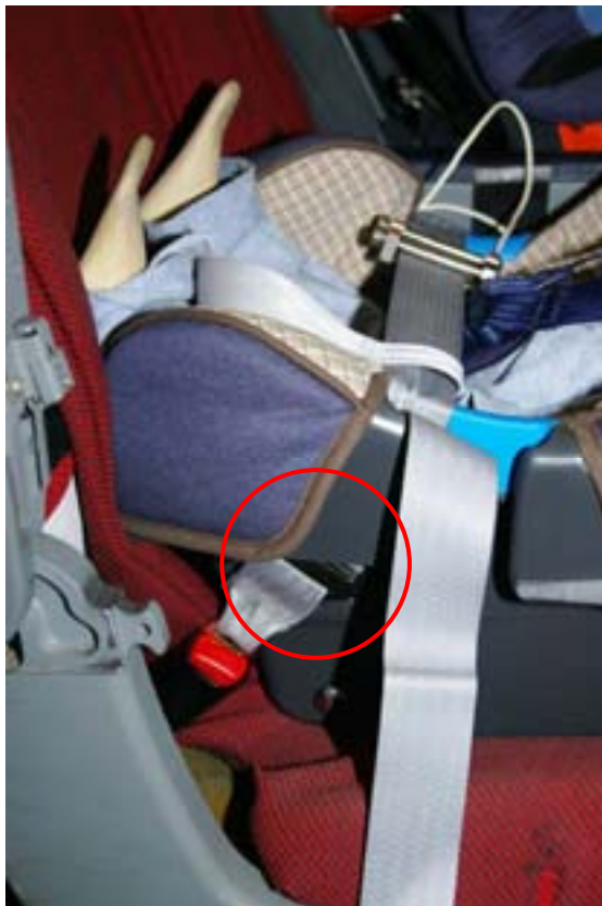
Figure 31- LATCH configuration for rearward facing CRS - Note adjuster positioned under guide
