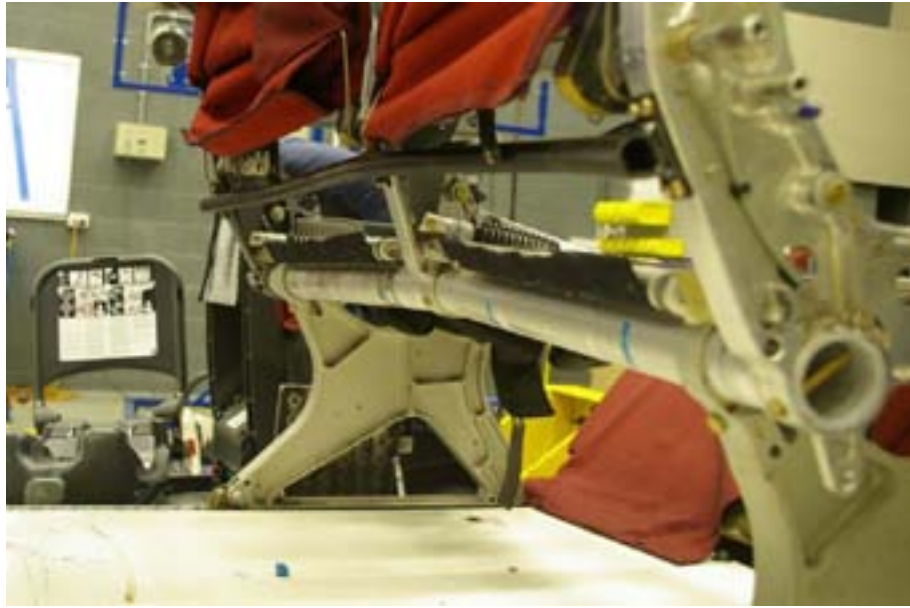
Figure 97 - Integrated Lower Anchorage (post-test 09-06)
