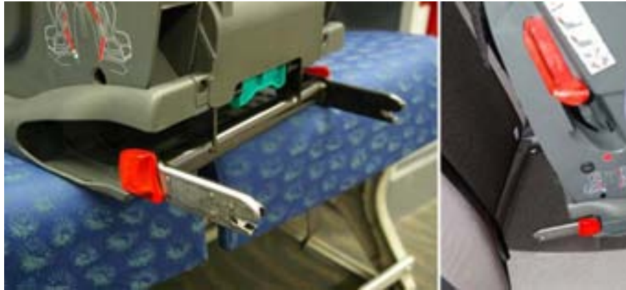
Figure 2 - A typical ISOfix child restraint anchorage system | Positioned ready for engagement in a car
