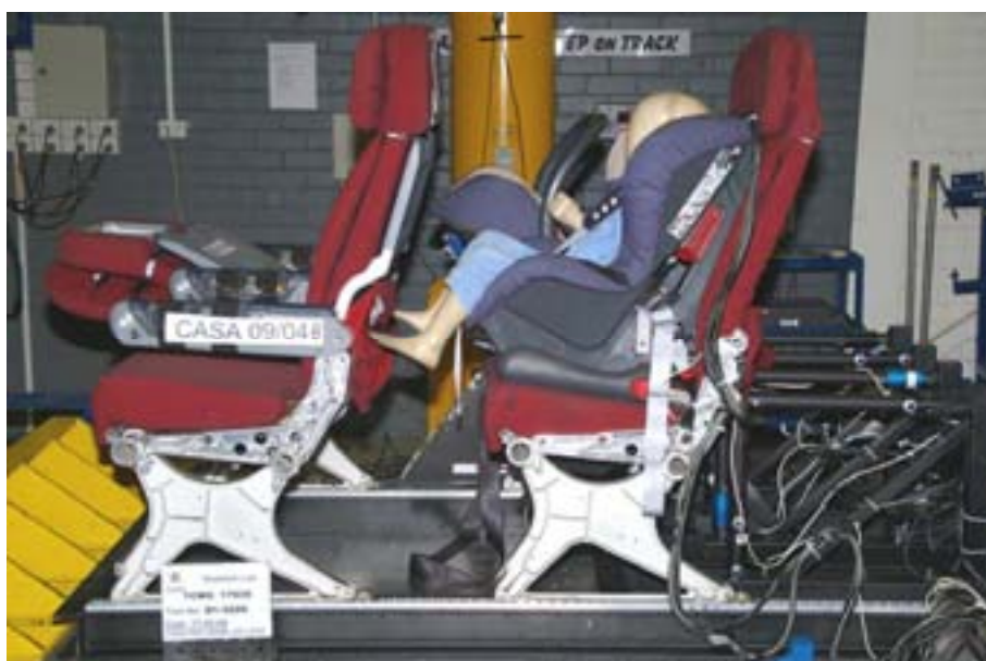
Figure 29 - Configuration tested - LATCH
