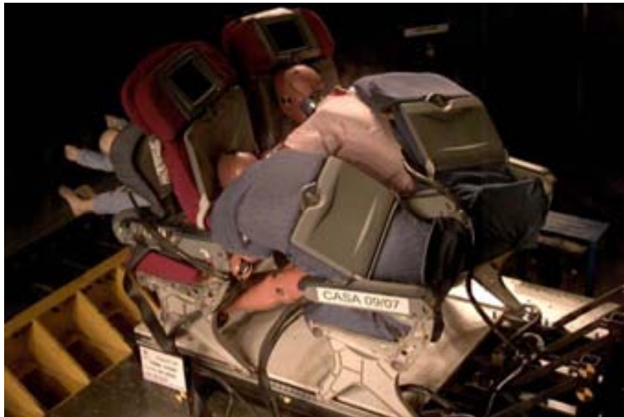
Figure 53 - Relative head strike placements @ 105ms
