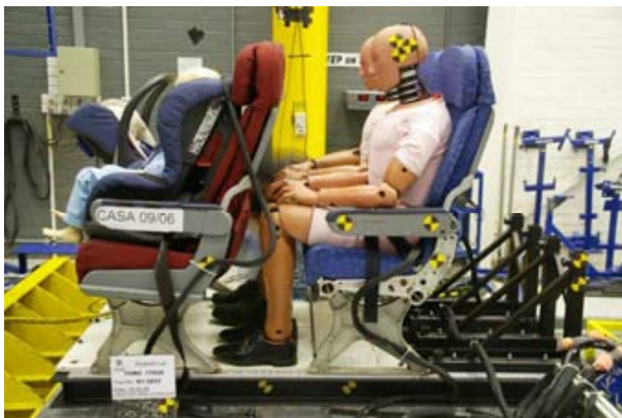
Figure 43 - Configuration tested - ISOfix with 50th percentile rear occupants
