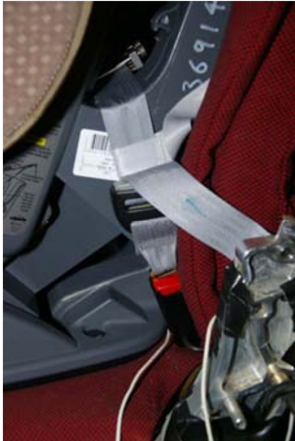
Figure 25 - LATCH configuration for forward facing CRS
