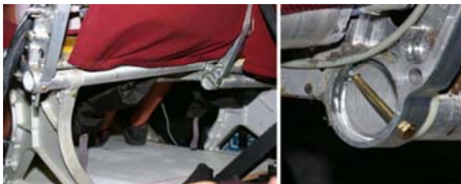
Figure 62 - Post test seat crossmember fracture (Adult ATD)
