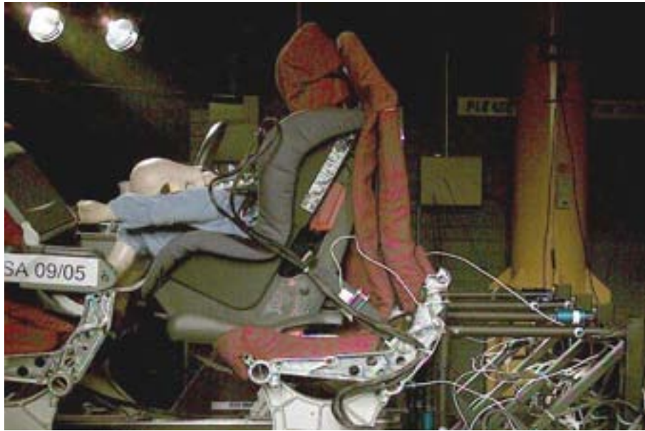
Figure 39 - P3 Maximum Head Excursion and Head strike on thighs @ 107ms
