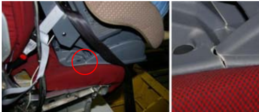
Figure 65 - RHS CRS Fractured Seat Base
