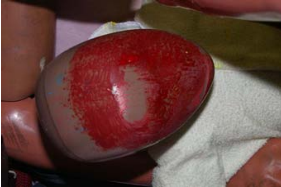
Figure 81 - P1½ head strike witness mark
