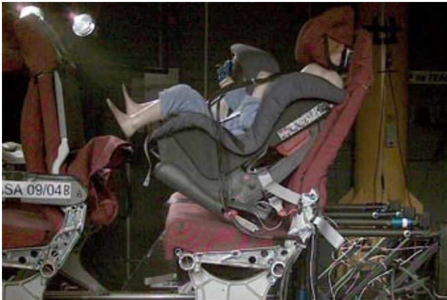
Figure 33 - P3 2nd Head strike on headrest @ 273ms
