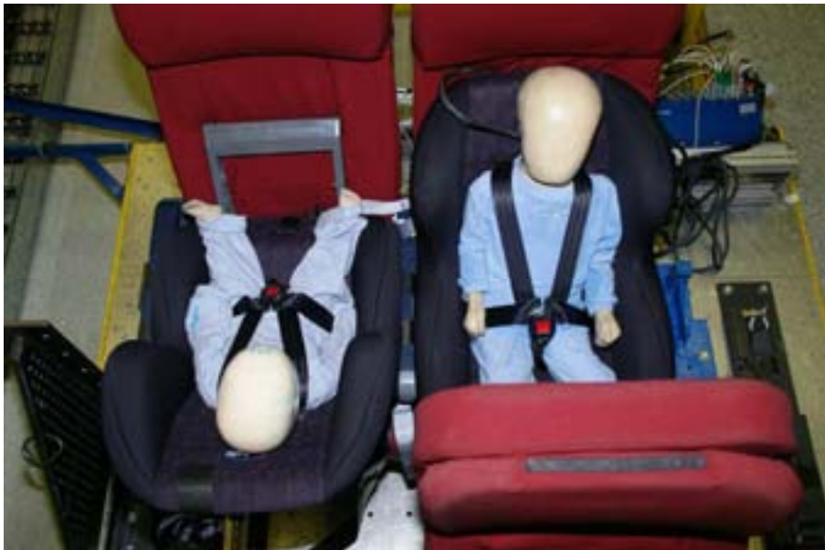
Figure 18 - Configuration tested - LATCH
