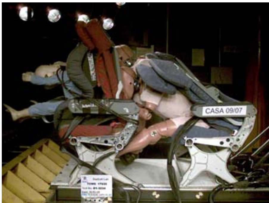
Figure 52 - Maximum seat back breakover @ 101ms
