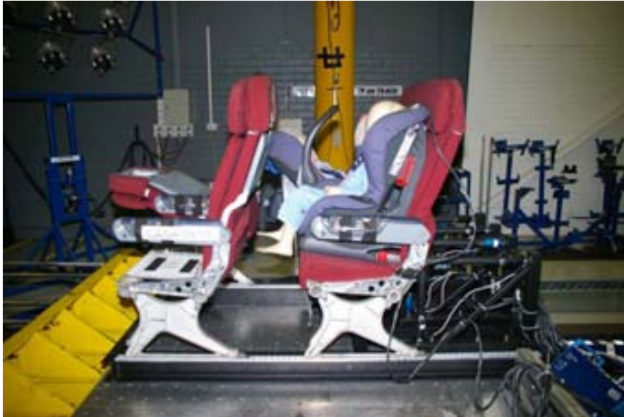
Figure 13 - Configuration tested - ISOfix
