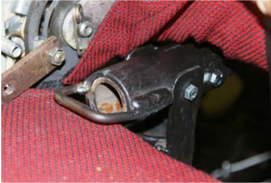
Figure 36 - Lower Anchorage post-test - Note upward bend to the 6mm loop
