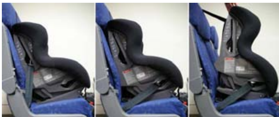
Figure 1 - IGC Alternate belt path | IGC Standard belt path | Unstable nature of forward belt paths without effective top tether.
