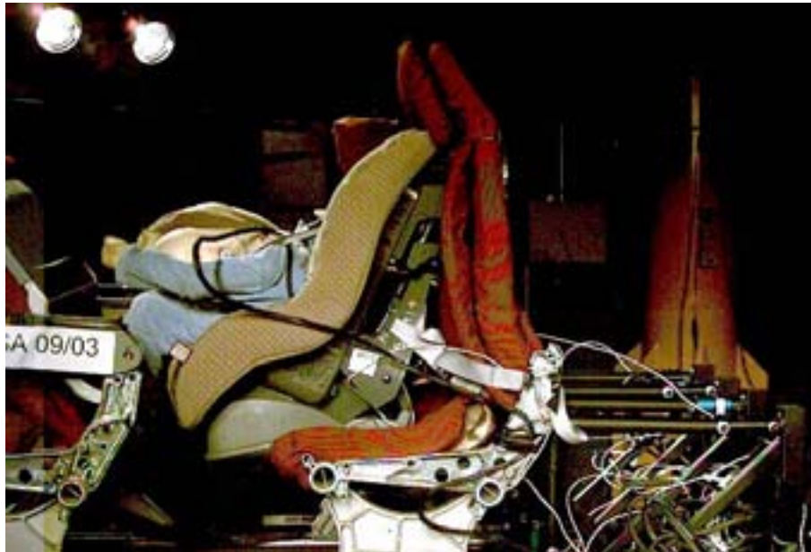
Figure 27 - P3 Maximum Head Excursion and Head strike on thighs @ 107ms
