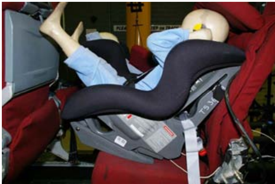
Figure 22 - Post Test, note CRS rotation and bunching of LATCH strap
