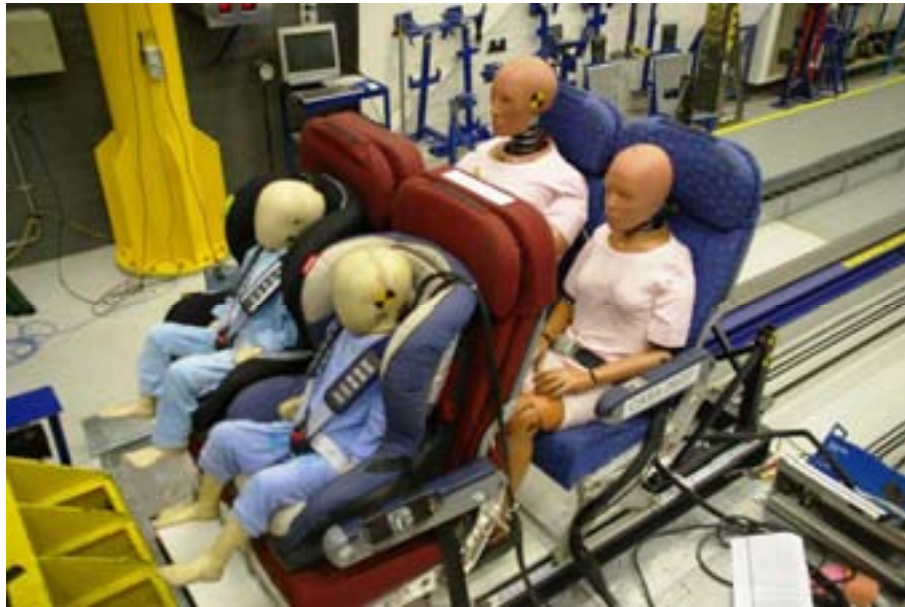
Figure 51 - Configuration tested - ISOfix with 5th percentile female and 95th percentile male rear occupants
