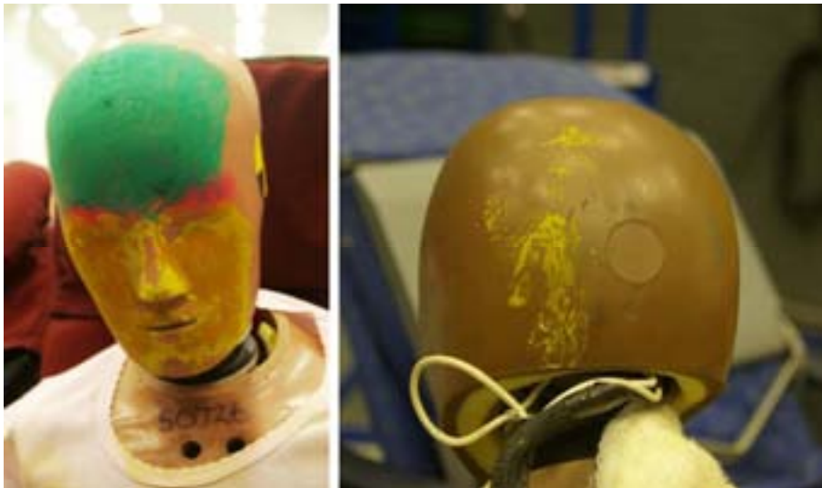
Figure 82 - Adult to P1½ Head Strike Paint Transfer, note adult forehead is clear of markings.
