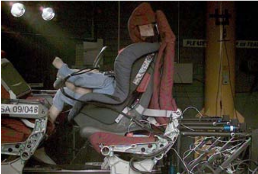
Figure 32 - P3 Maximum Head Excursion and Head strike on thighs @ 107ms
