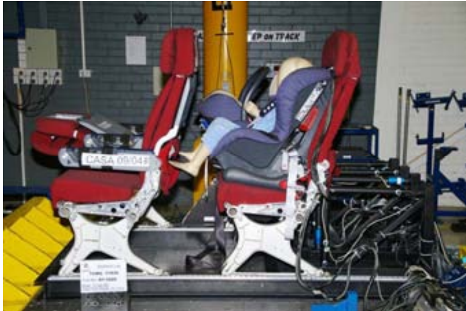
Figure 6 - Seating configuration for Lower Anchorage Loads gathering
