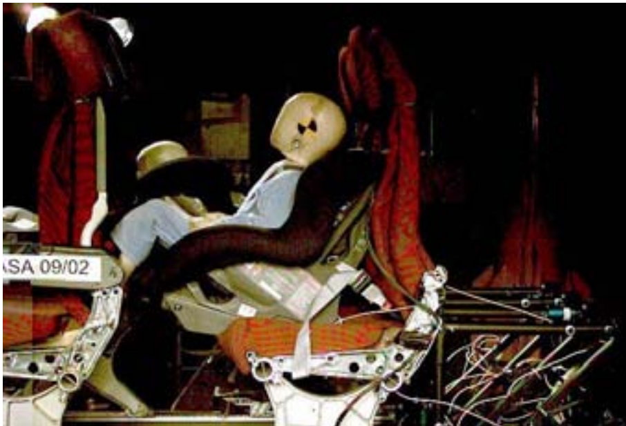
Figure 20 – P3 Foot engagement @ 60 ms - Note high knee position due to reclined CRS
