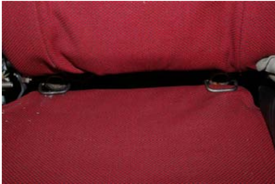
Figure 94 - Lower Anchorage Loops protruding through seat bight.
