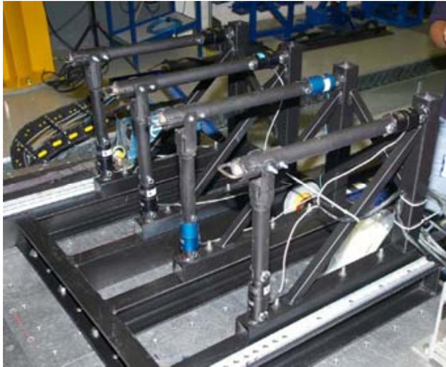
Figure 92 - Instrumented Lower Anchorage arrangement
