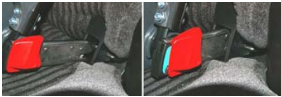
Figure 3 - ISOfix attachment lined up in a guide for engagement | Green marking indicating successful attachment.
