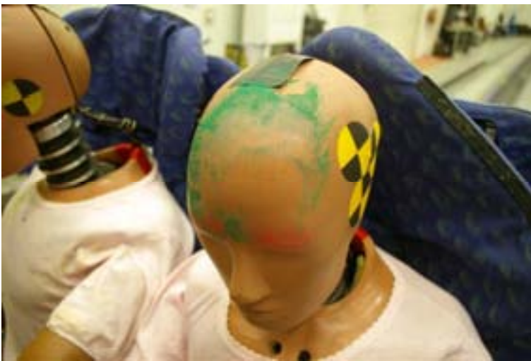
Figure 48 - Seat back damage - LHS tray table, RHS tray table, LHS Adult ATD head witness mark - Note the different vertical placement of witness marks on tray tables.
