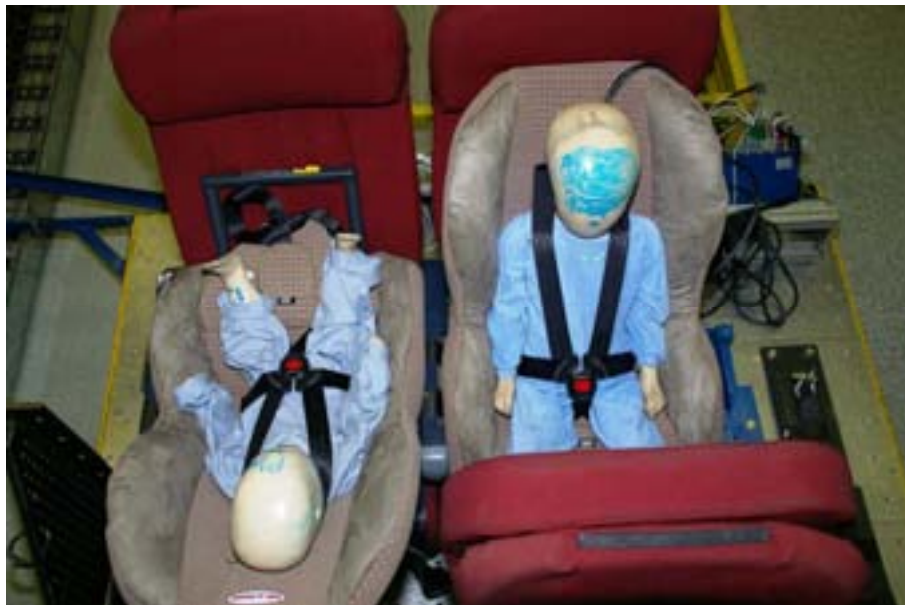
Figure 24- Configuration tested - LATCH
