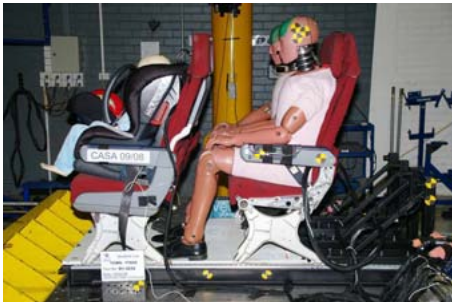
Figure 59 - Configuration Tested - lap belt restrained CRS
