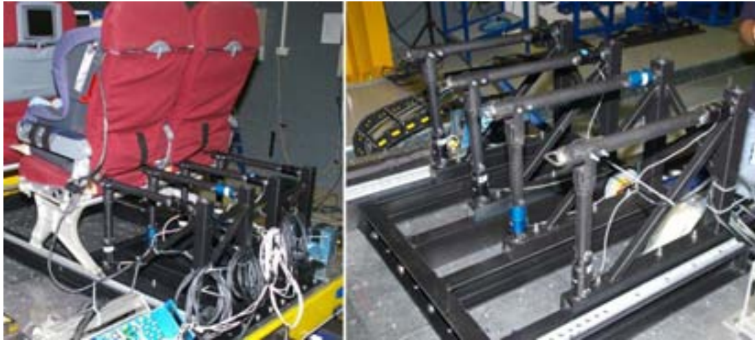
Figure 7 - Instrumented Rigid Lower Anchorages
