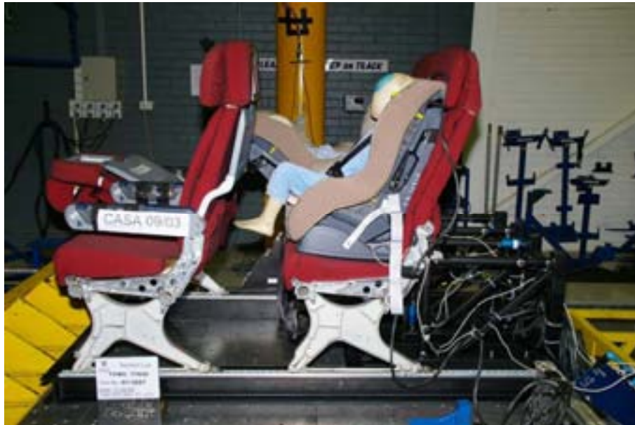
Figure 23- Configuration tested - LATCH
