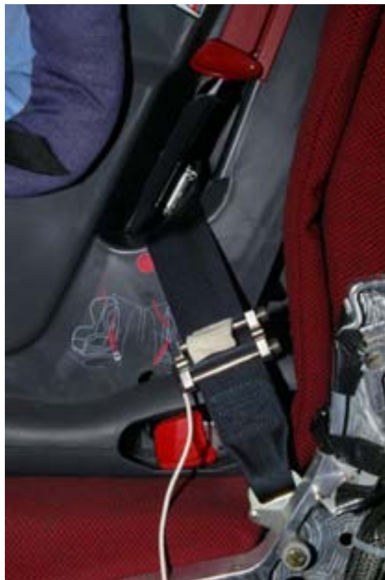
Figure 38- Lap Belt configuration for forward facing CRS
