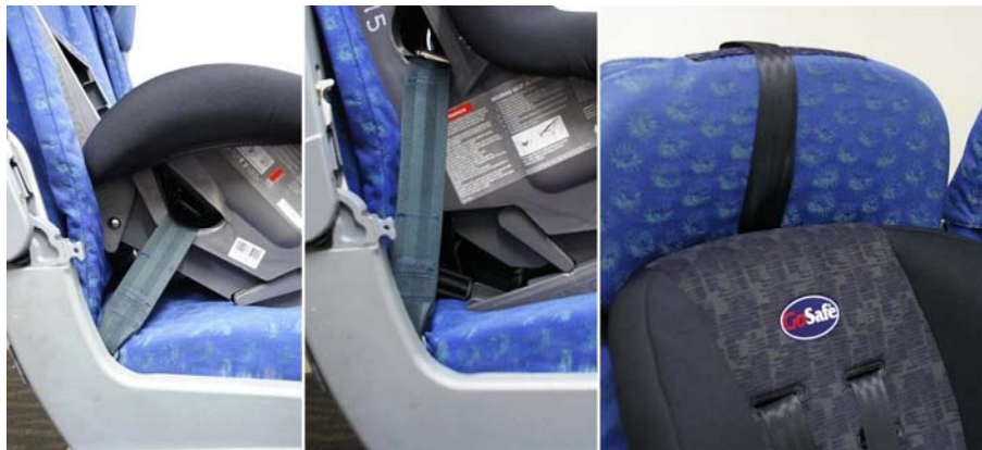
Figure 7 - Belt Angles - Rear facing | Forward facing | Forward facing top tether
