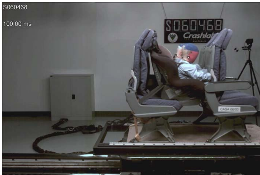
Figure 20 - Maximum displacement of Gosafe CRS
