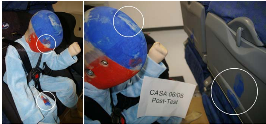
Figure 26 - Witness marks of head strikes on the knee and tray table
