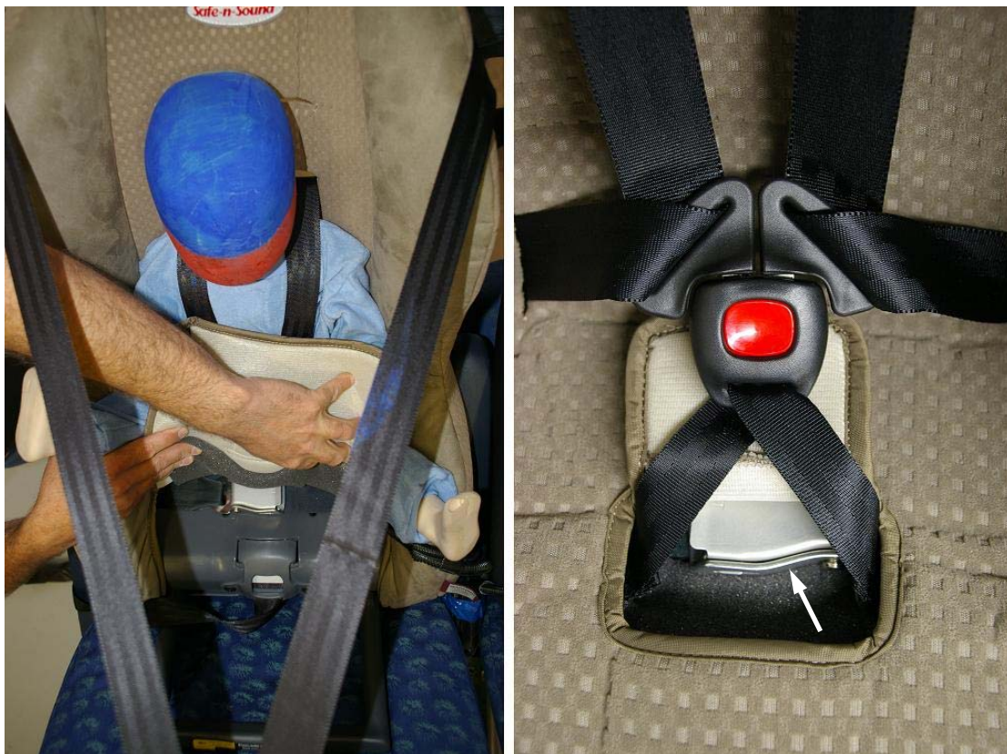
Figure 39 - Buckle position on the Safe-n-Sound in rear facing mode
