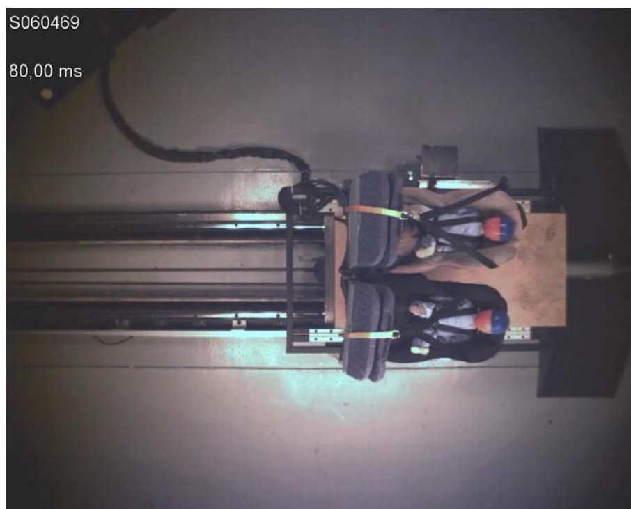
Figure 16 - Maximum horizontal head protrusion
