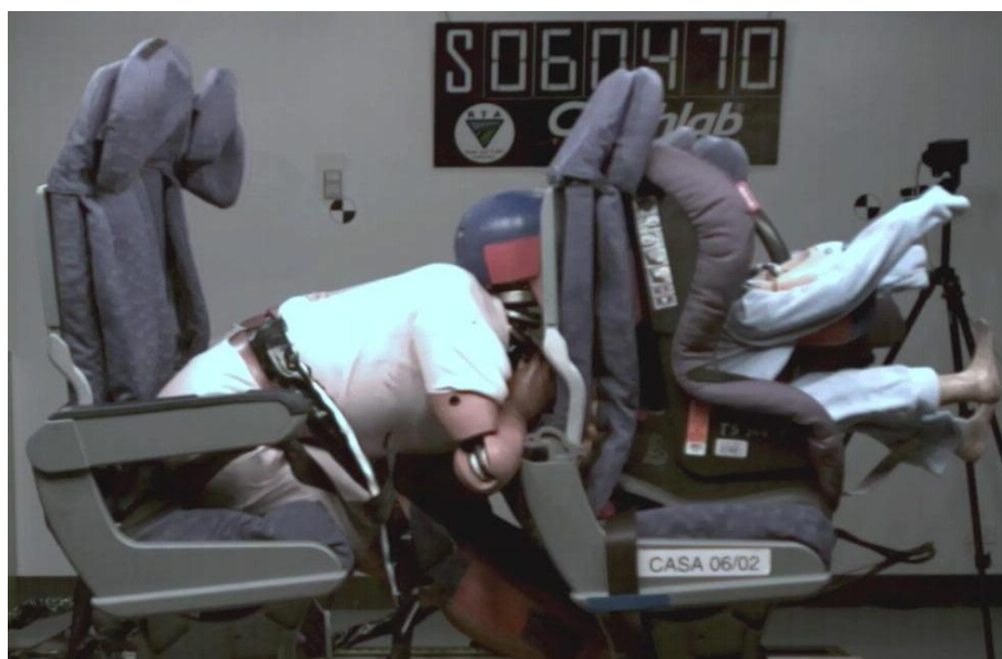
Figure 10 – ISOfix CRS potential interference with injury levels for adults seated behind - Point of maximum head rotation for the Hybrid III ATD
