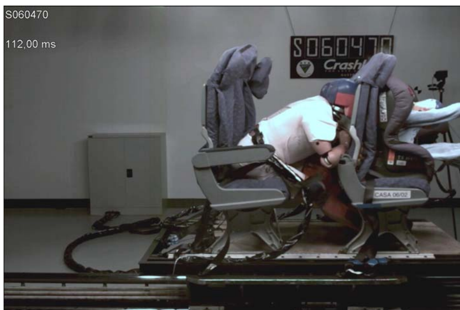
Figure 32 - Point of maximum seat back break over and maximum P3 head excursion
