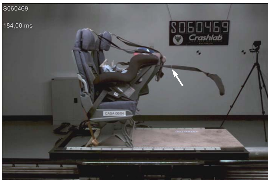
Figure 18 - Sock whip. Note strap adjustment chalk mark (arrowed)
