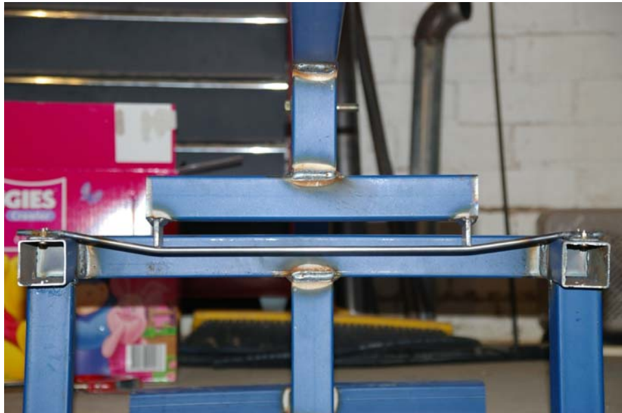
Figure 47 - Prototype lower anchorage showing permanent set after load application
