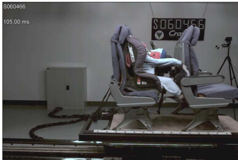
Figure 28 - Maximum head excursion of the P3 ATD and forward facing CRS
