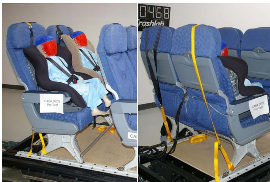
Figure 19 – Note vertical orientation of top tether to CRS | note also different styles of CRS top tether (single strap vs. V arrangement) and method of top tether anchorage to seat.
