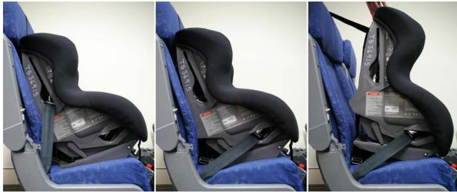
Figure 4 - IGC Alternate belt path | IGC Standard belt path | Unstable nature of forward belt paths without effective top tether.
