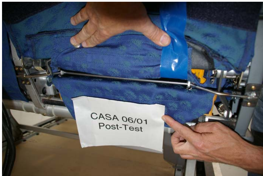
Figure 30 - ISOfix lower anchorage bent by the P3 ATD and forward facing CRS
