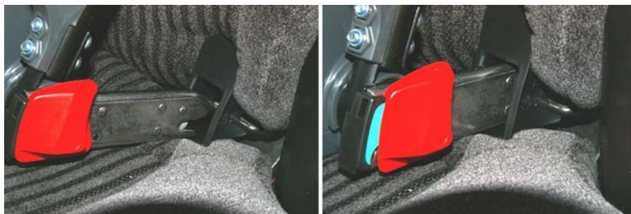
Figure 3 - ISOfix attachment lined up in a guide for engagement | Green marking indicating successful attachment.
