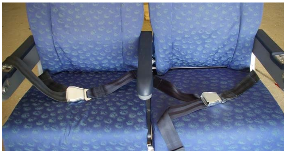
Figure 46 - The seat on the left shows the lower anchorage covered by upholstery | The seat on the right shows the lower anchorage revealed.
