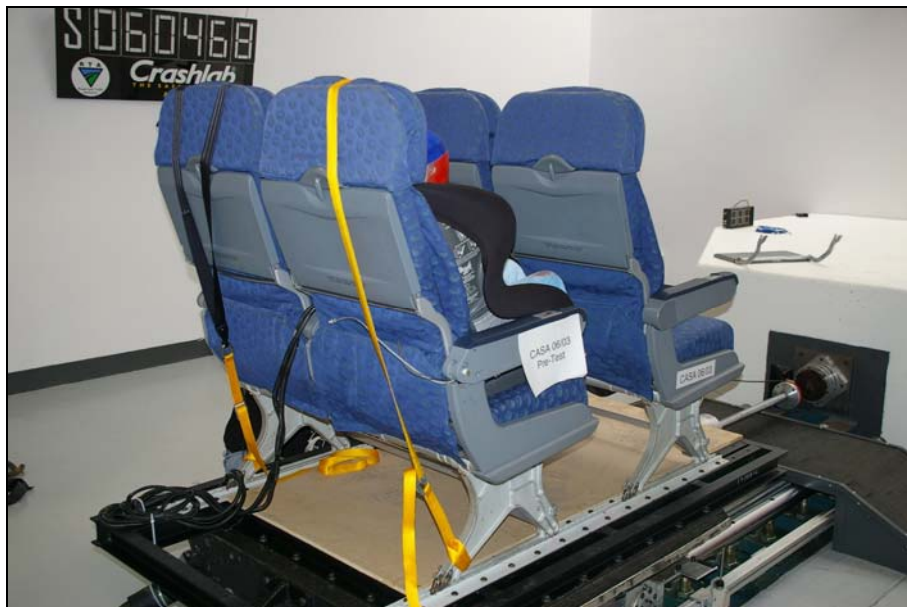
Figure 1 – Typical top tether installation with strap across tray table
