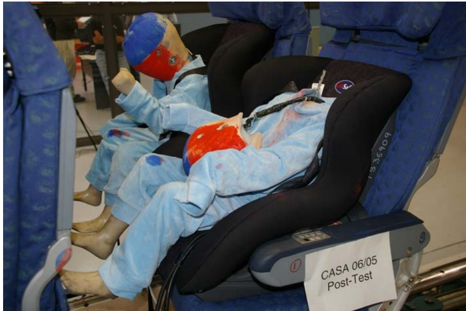
Figure 24 – Post-test showing head attached only by instrumentation wiring. The broken spinal cable can be seen protruding from the neck region.
