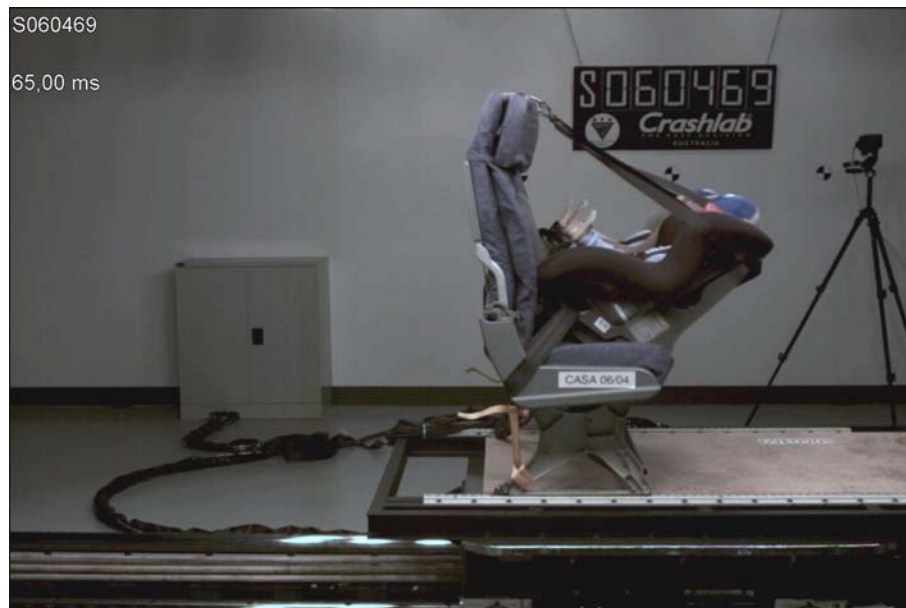
Figure 15 - Maximum Gosafe head protrusion
