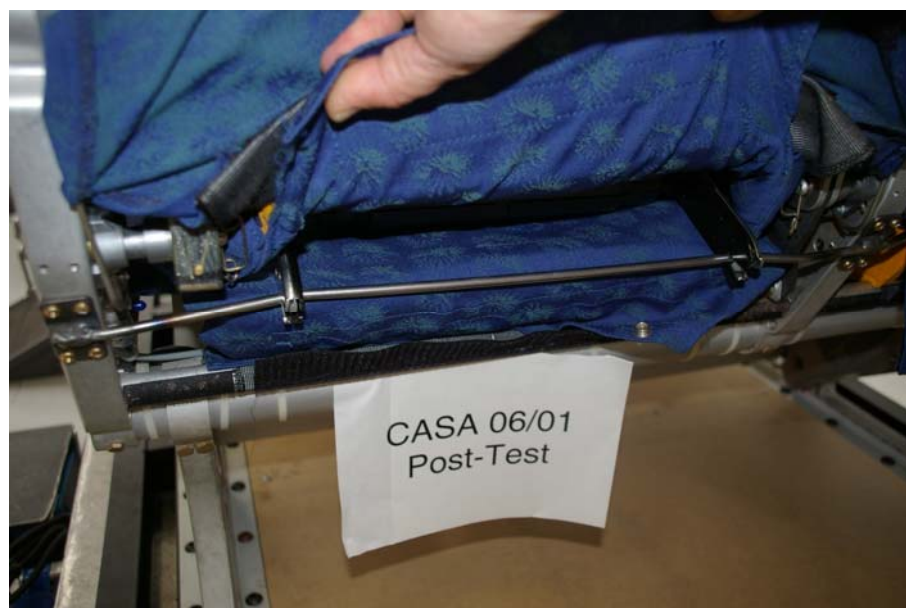
Figure 29 - ISOfix lower anchorage bent by the P3/4 ATD and rear facing CRS
