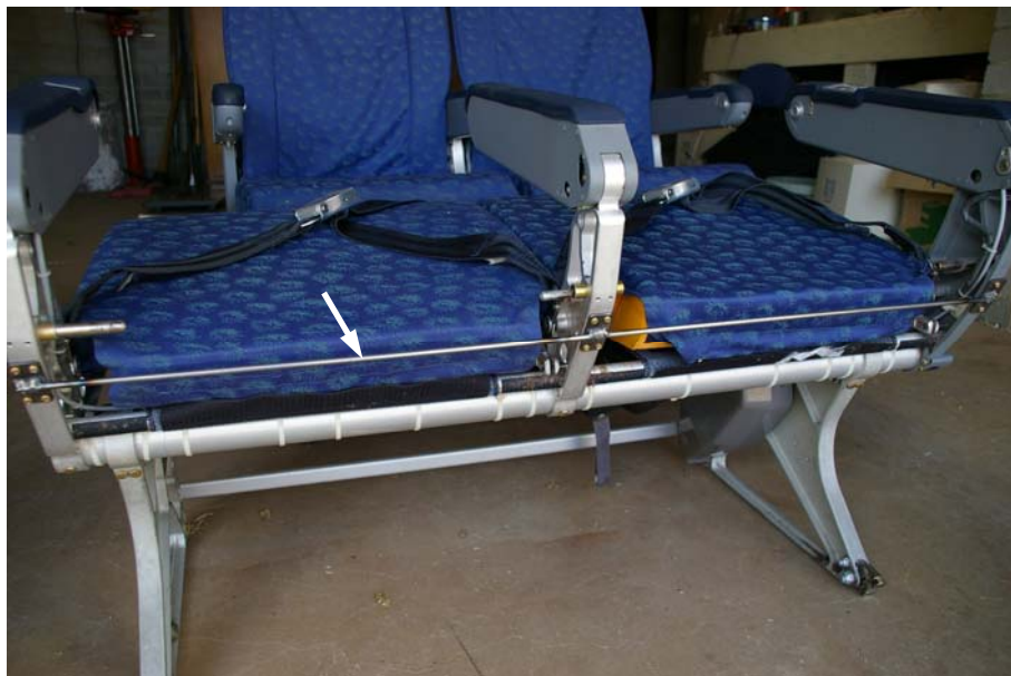
Figure 43 - ISOfix lower anchorage installation (seat back sub-assemblies removed)
