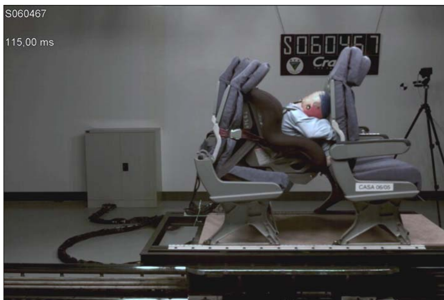
Figure 25 - Point of maximum head excursion, prior to knee contact.
