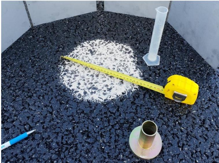
**Figure 5. Sand patch test.**
