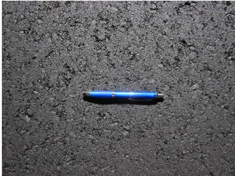
**Figure 3. Surface texture of typical ungrooved airport DGA.**
