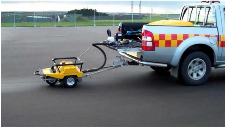
**Figure 6. Example Griptester CFME in operation.**
