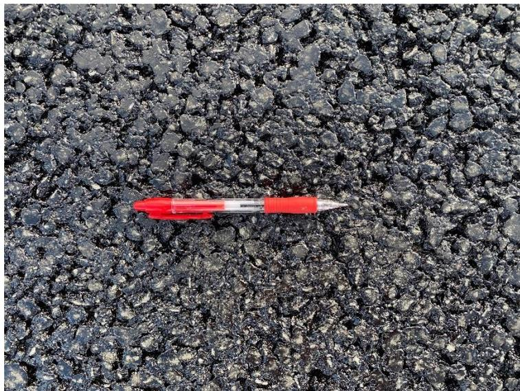
**Figure 4. Surface texture of typical airport SMA.**
