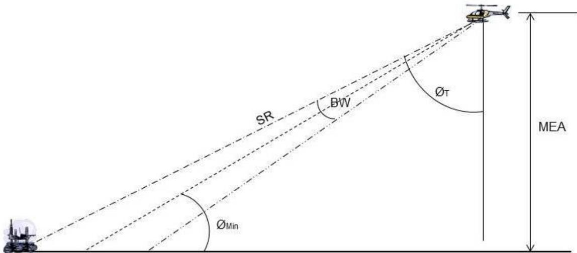
**Figure 1: Obstacle clearance descent profile**
