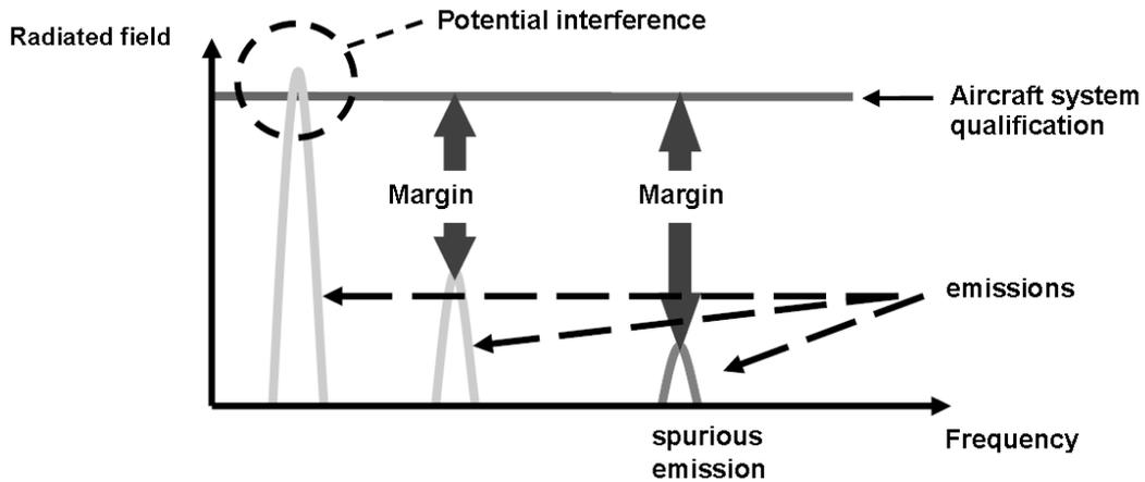
Figure 5: Backdoor coupling of radiated emissions
