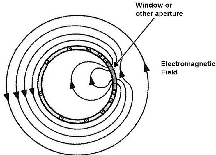
**Figure 10: Propagation of an electromagnetic field through a window or other aperture**
