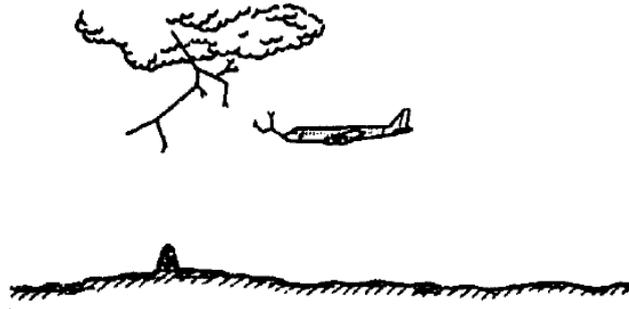
**Figure 9: Aircraft interaction with a lightning leader and streamer**
