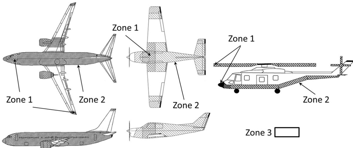
**Figure 14: Examples of aircraft lightning strike zones**
