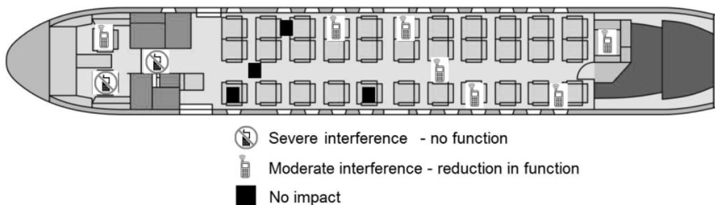
**Figure 6: Example of false smoke detection identified during mobile phone testing**
