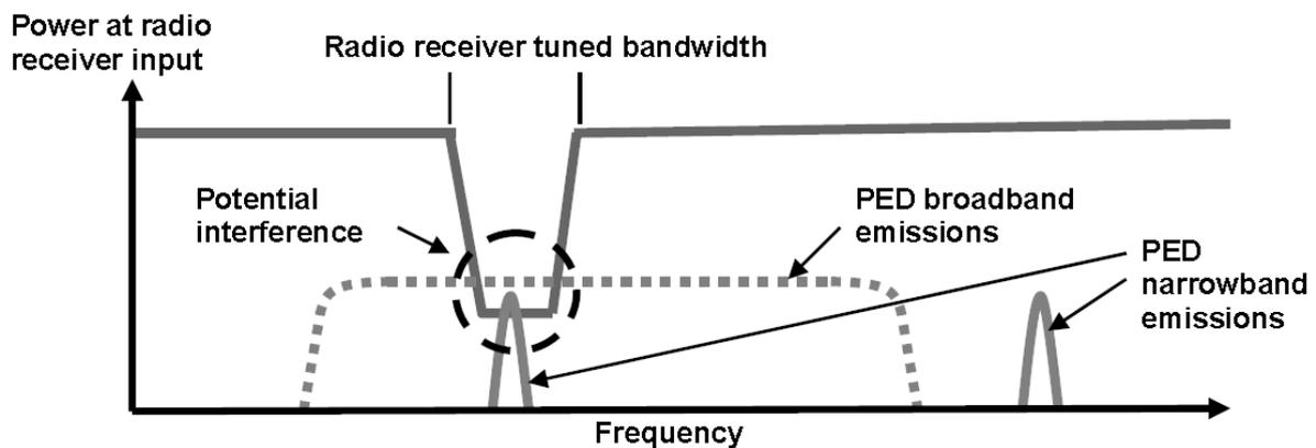
**Figure 7: Potential portable electronic device emissions to aircraft systems**
