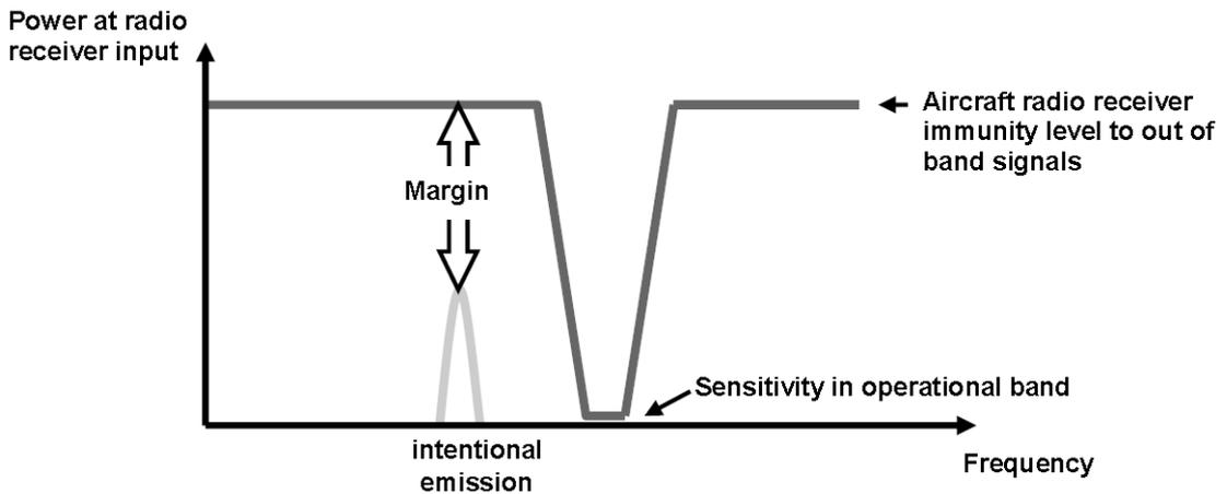
Figure 2: Front door coupling of intentional radiated emissions
