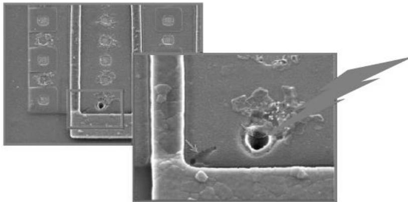
**Figure 12: Microprocessor damage by the indirect effects of lightning**
