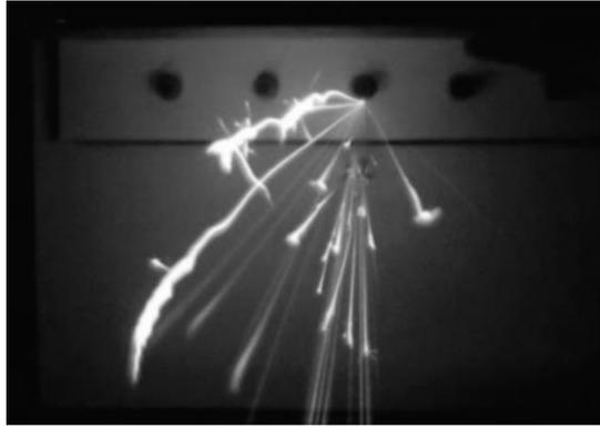
**Figure 11: Sparking rivets**
