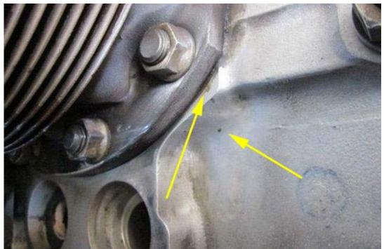
Figure 1 - Failure of a weld-repaired crankcase. Note crack from the cylinder base stud.
