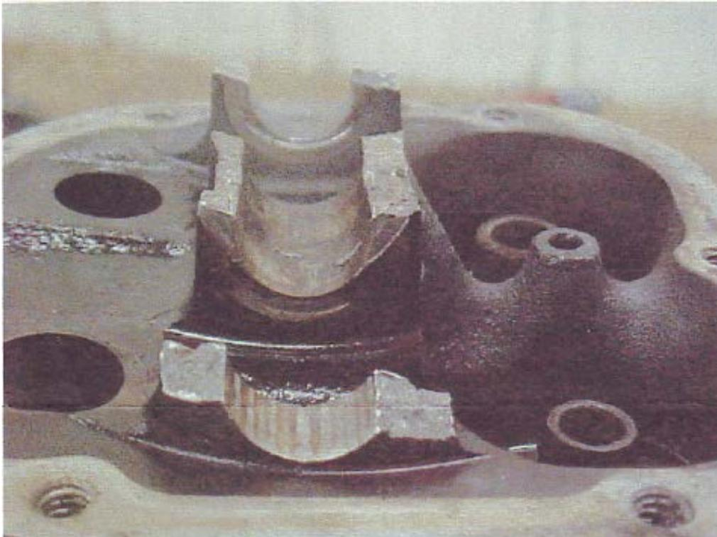
Many failures may be attributed to not following the engine manufacturer's overhaul and maintenance instructions and / or not following good overhauling component handling practices. The bosses are cast into the head and are susceptible to any shock loading.
