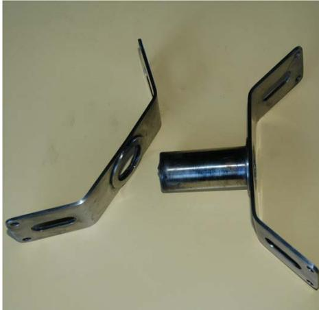
Figure 3: Failed burner gimbal mount
