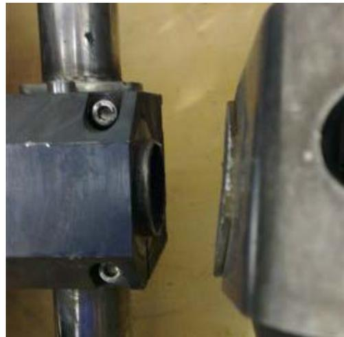
Figure 2: Close-up of weld-failure
