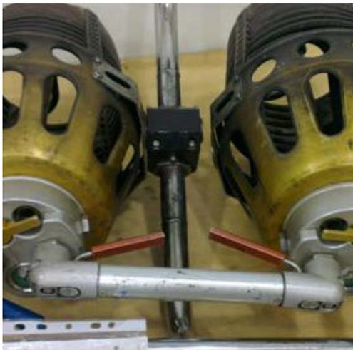
Figure 1: Double Stratus burner unit. Note dislodged burner on the right.
