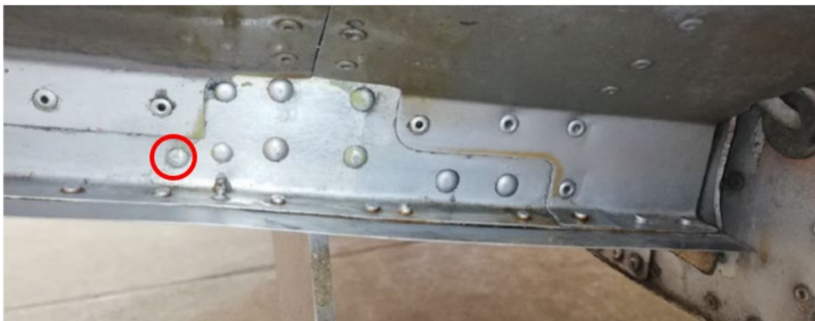
Figure 1: CAA NZ AD DCA/CT4/9 Critical Fastener Location Near Rear Spar Wing Root
