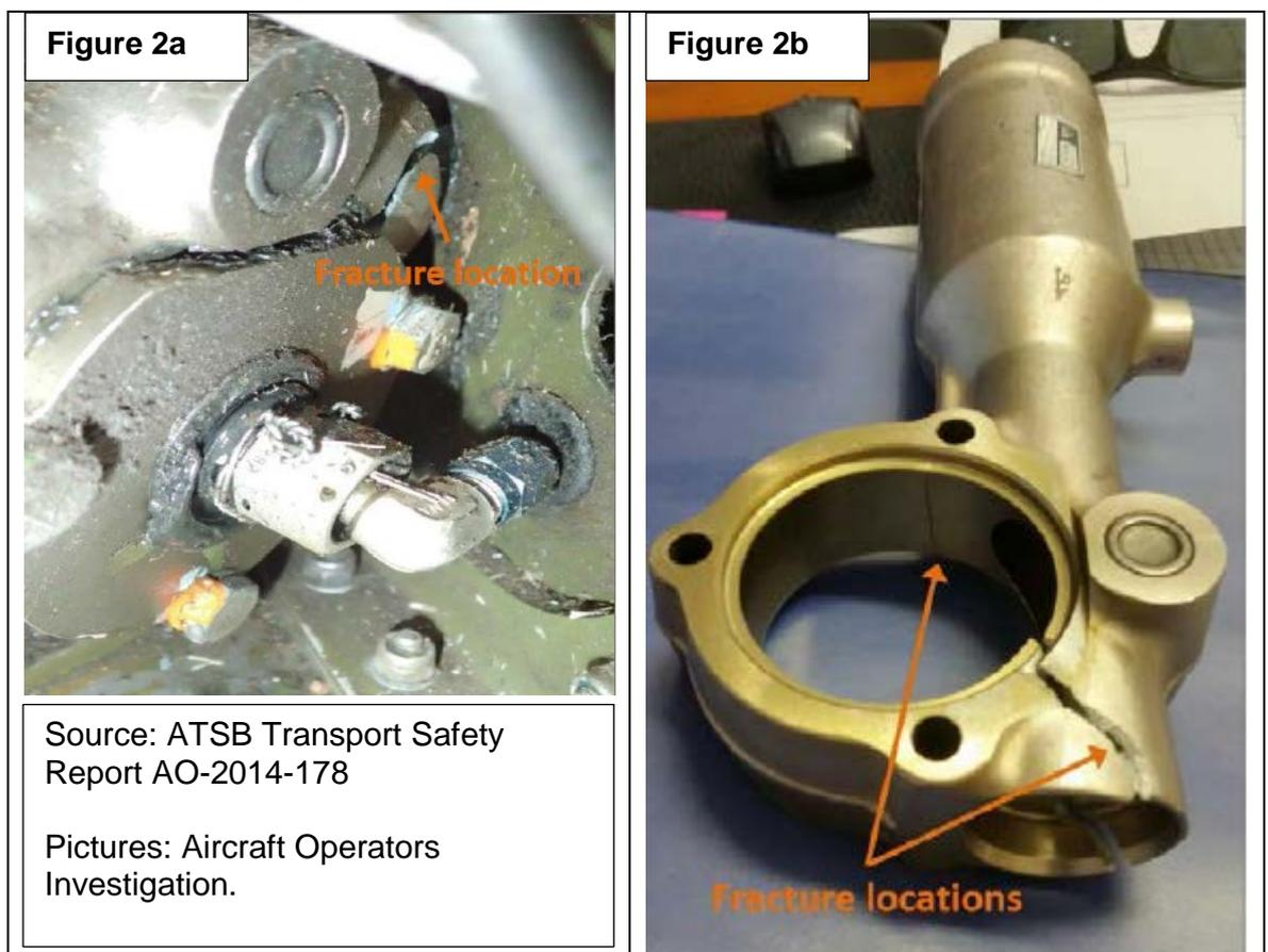
There have been other cases of Cessna single engine retractable aircraft where the main landing gear could not be either fully retracted or extended due to broken actuator piston rack teeth, or due to the housing cracking open, resulting in actuator disengagement.
