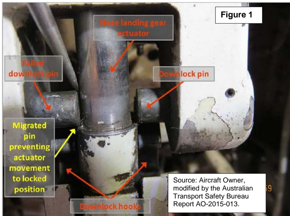
The old style nose landing gear down lock pins work loose, crack and fail at the retaining groove, which allows them to move out and jam the undercarriage actuator. This prevents the nose landing gear from locking fully down. The nose gear typically collapses on landing. ATSB report AO-2015-013 reflects that the US National Transport Safety Board (NTSB) has received over 30 reports of failed nose landing gear down lock pins.
