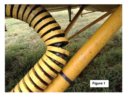
Previous technical assessments of identical failures came to the conclusion that adverse wear on the internal structural tube could not be detected using the manufacturer's maintenance data, or by the requirements of CASA Schedule 5.
