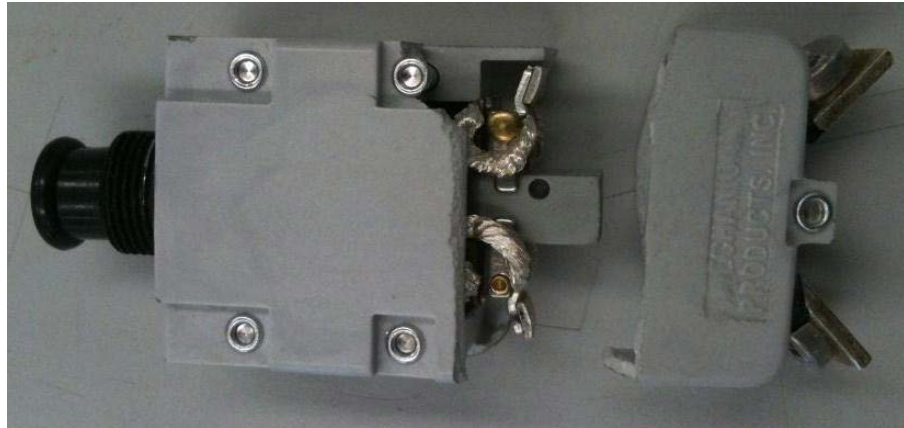
Figure 5 – Propeller Auxiliary feather CB damaged by placement on panel
