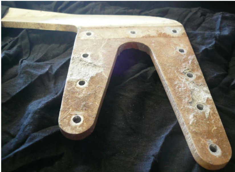
Figure 4. Corroded section of flap hanger bracket.
