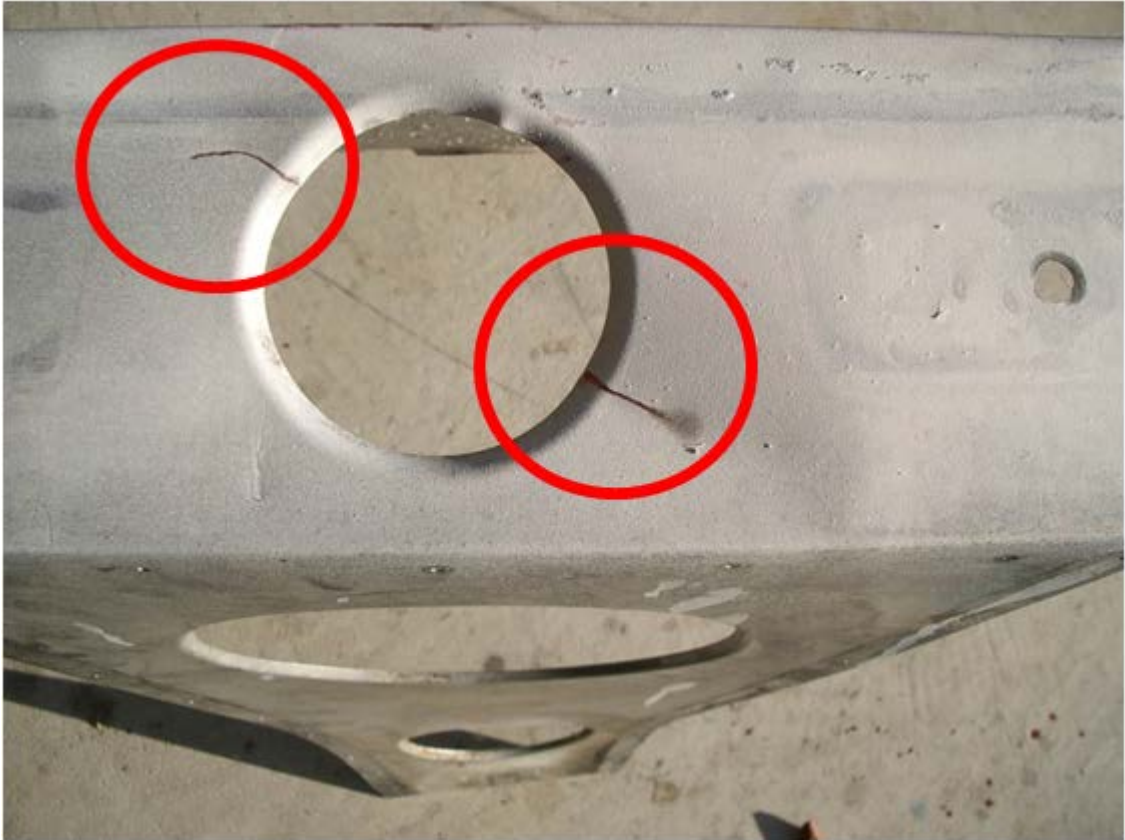
Cessna 172 Horizontal Stabilizer Front Spar Cracking
