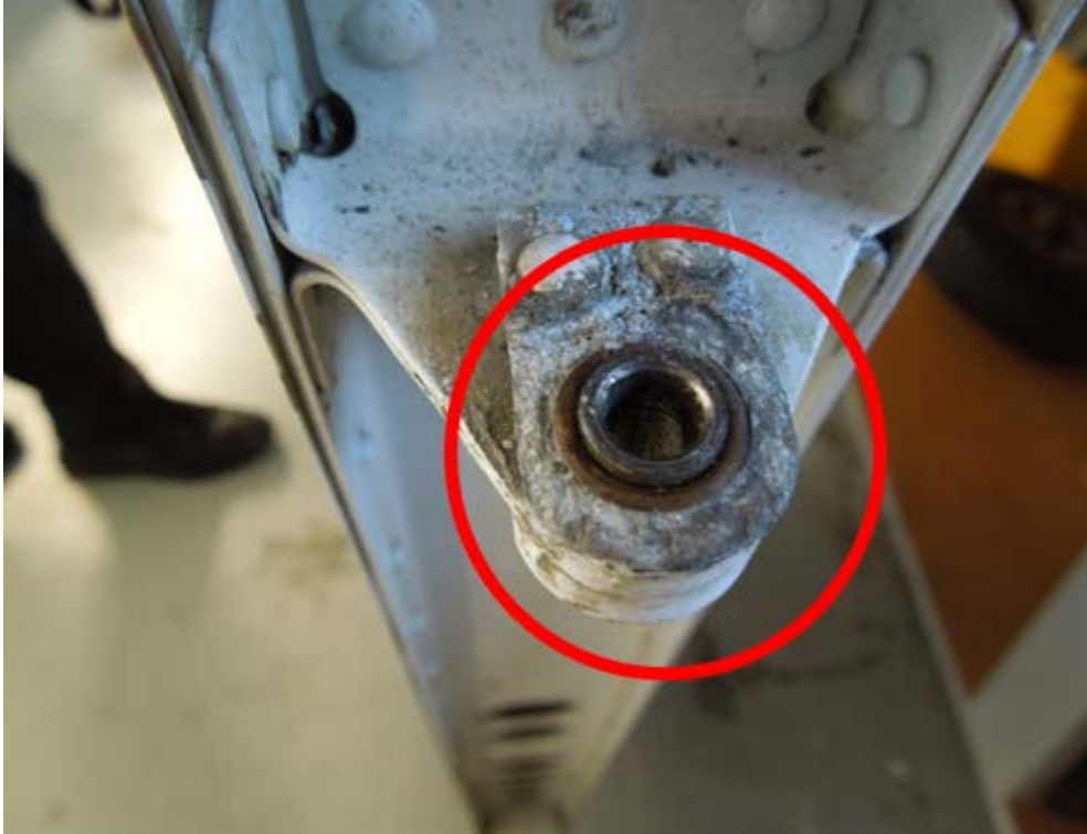
Centre Rudder Hinge Mount Corrosion
