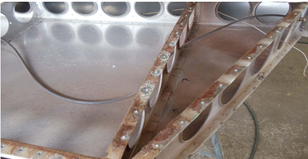
Cessna 152 vertical fin corroded under the skin of the fairing
