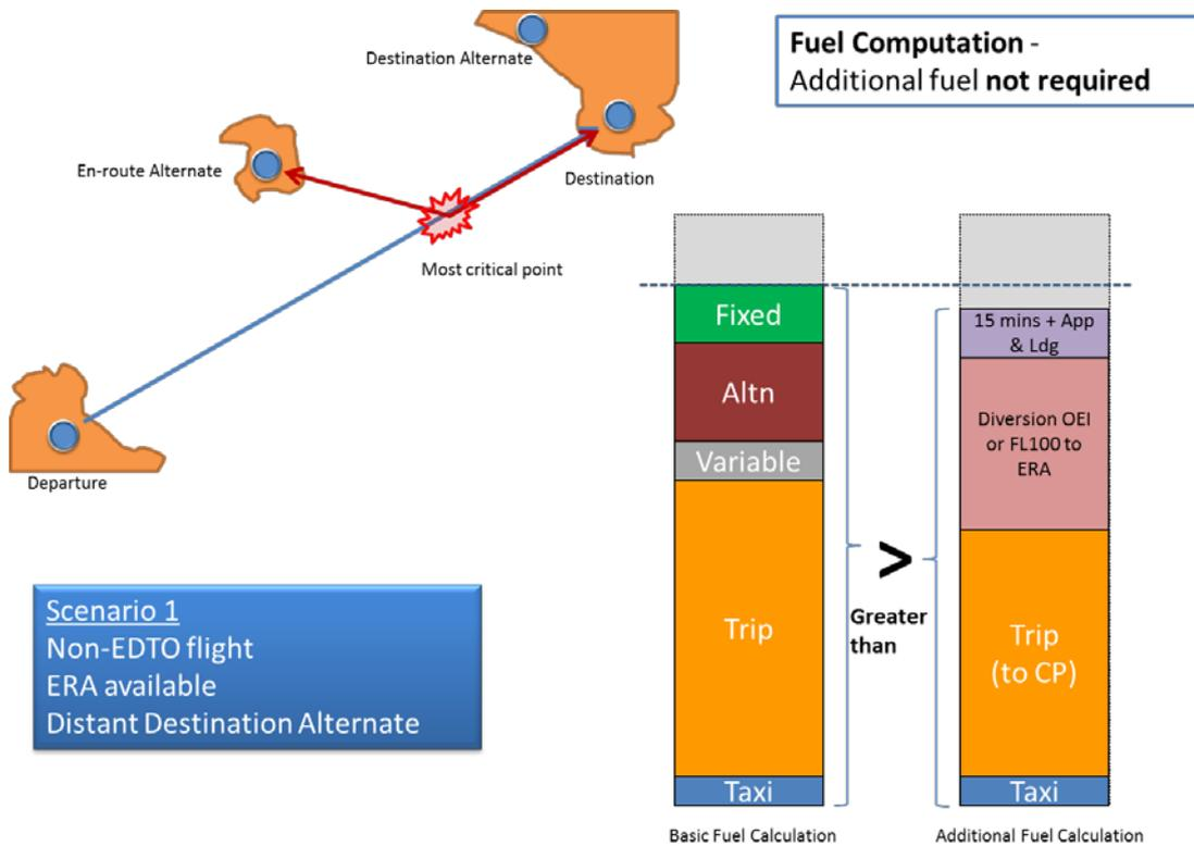
Figure 2: Fuel calculation scenario – additional fuel not required
