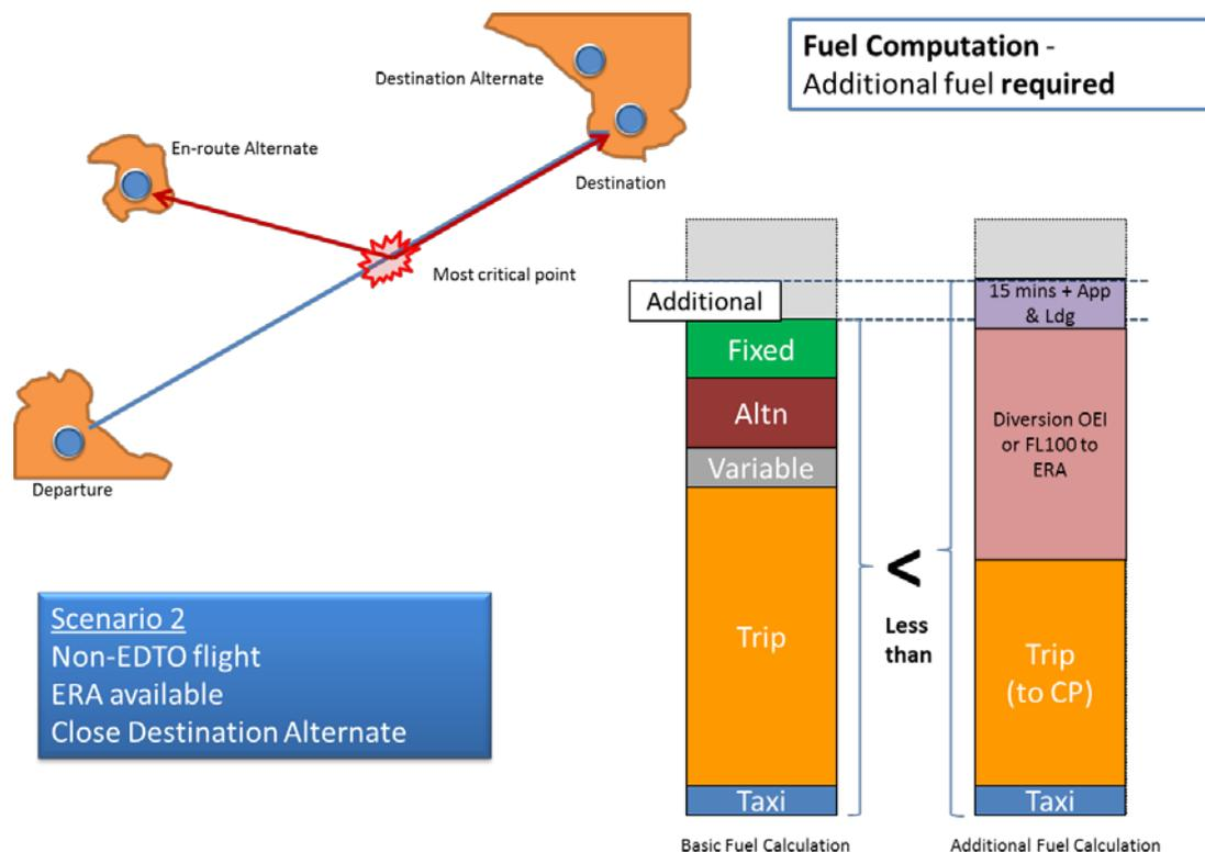
**Figure 3: Fuel calculation scenario –additional fuel required**
