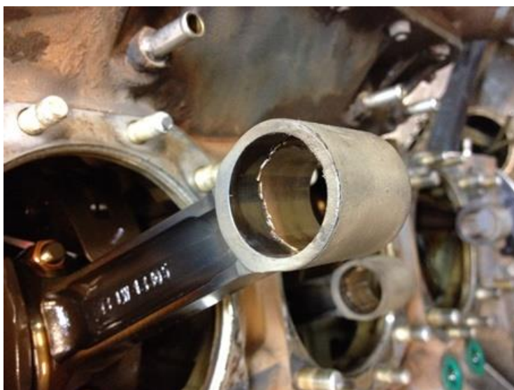
Figure 4 -Partially disassembled O-540-F1B5 engine with an accumulated Time Since New from September 2011 of 1031 Hours, showing material loss and breakup of the connecting rod little end bush. Four (4) of the six (6) bushes from this engine had varying degrees of material loss.
