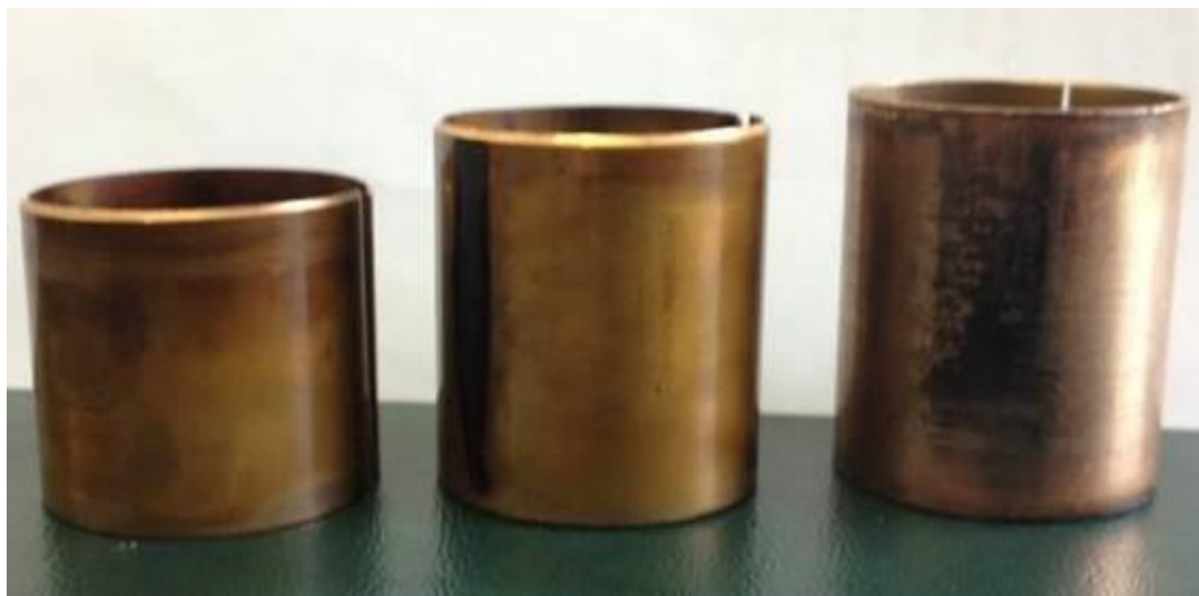
Figure 3 - Three (3) P/No LW13923 Bushes from an O-360-J2A engine which had accumulated 1000 Hours since rebuild in September 2011, showing varying degrees of abrasive wear and consequential reduction in bush axial length. The bush on the right has a relatively unworn axial length.
