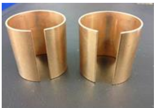
Figure1 - The bush on the right is a Connecting Rod Small End Bush P/N LW-13923, identifiable by the pre-set split line which is almost twice the width of the bushing previously received from Lycoming, shown on the left.
