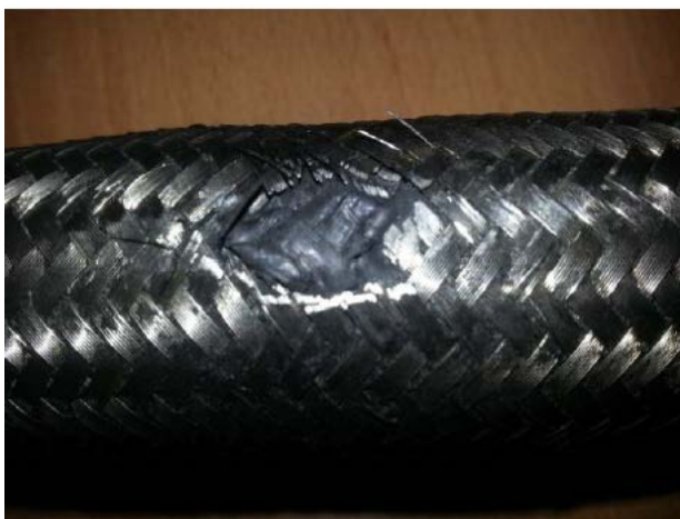
Hose (above) failed due to chafing against the structure (right).
