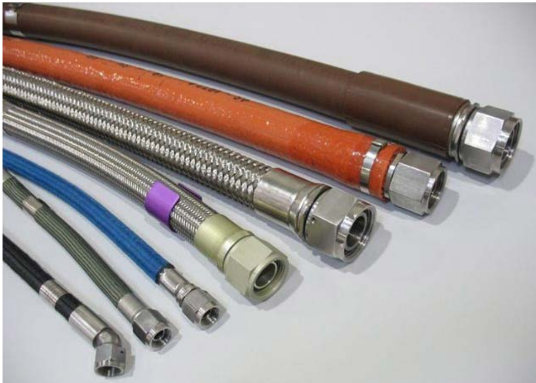
Figure 1. Aircraft use many different types of flexible hose, and each hose type has specific maintenance requirements. (Picture: Eton Hoses)
