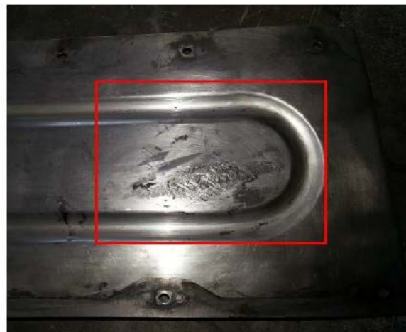
Hose (above) failed due to chafing against the structure (right).
