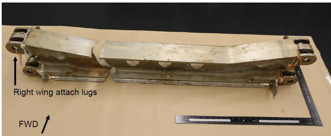
Figure 2: Photograph of Cessna T210M Fractured Carry-Thru Spar. View looking AFT at lower chord surface. Photo: ATSB AO-2019-026 Preliminary Report
