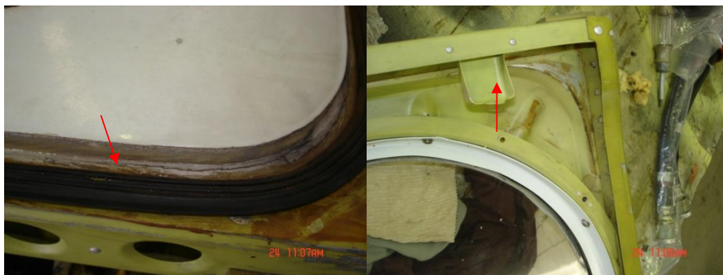
Figure 1. This aircraft contained a crack in the door structure that was detectable from the outside.
