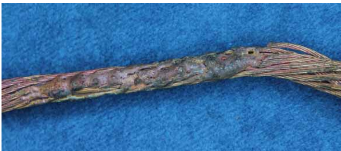
Figure 3 – Heat damage to DC input wire
