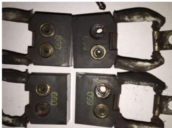
Figure 8 - Loose starter/generator brush rivets
