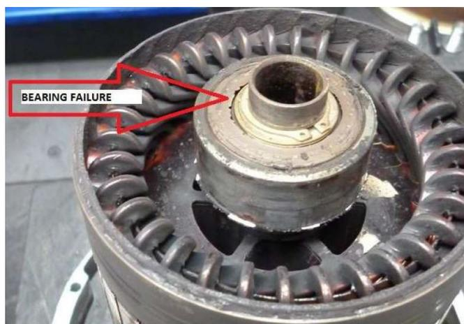
Figure 4 - Bearing failure
