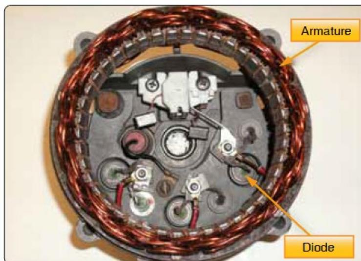
Figure 9 – Alternator diodes
