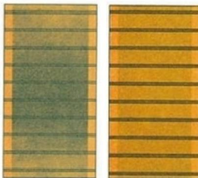
Figure 5 - Out of round compared to good condition commutator
