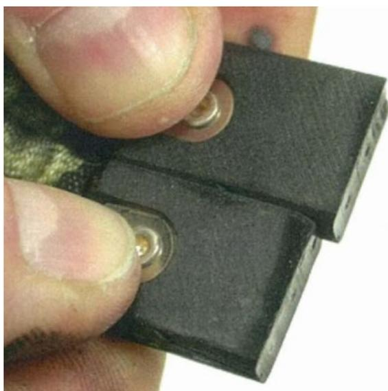
Figure 7 - Uneven Starter/generator brush wear rates
