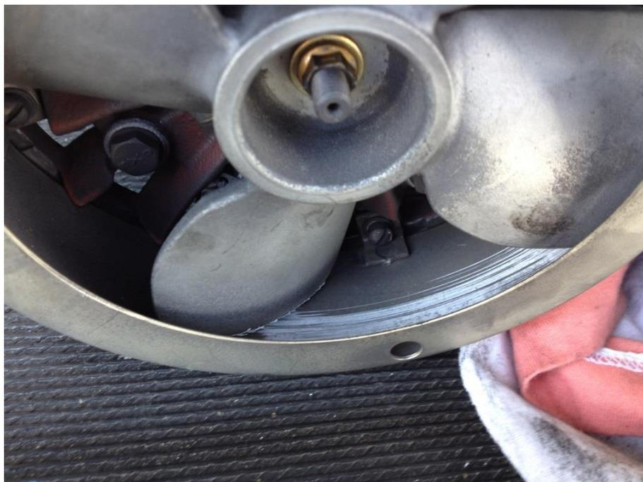
Figure 2 – Starter/Generator fan damage due to bearing failure
