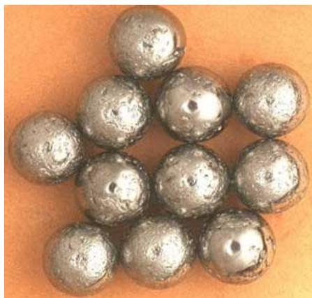
Figure 3 – Spalling damage
