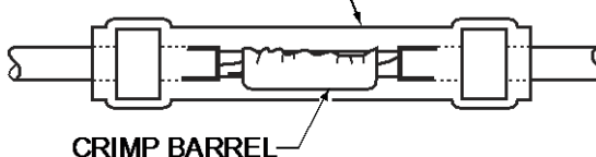
Figure 5-13 Sealing Sleeve Centred Over Crimp Barrel
