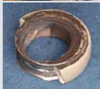
Bottom photo - pitch change link - Courtesy of the ATSB
