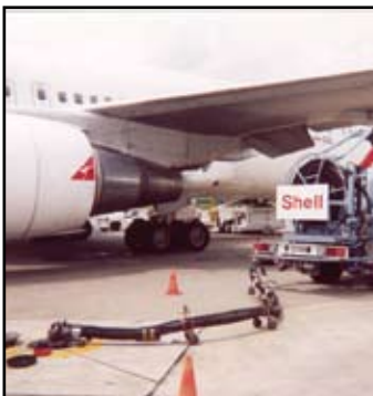
Refuelling aircraft with a hydrant dispenser
