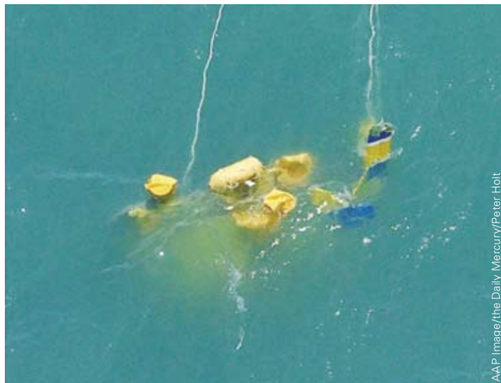
Flotation devices attached to the helicopter wreckage assist recovery.
