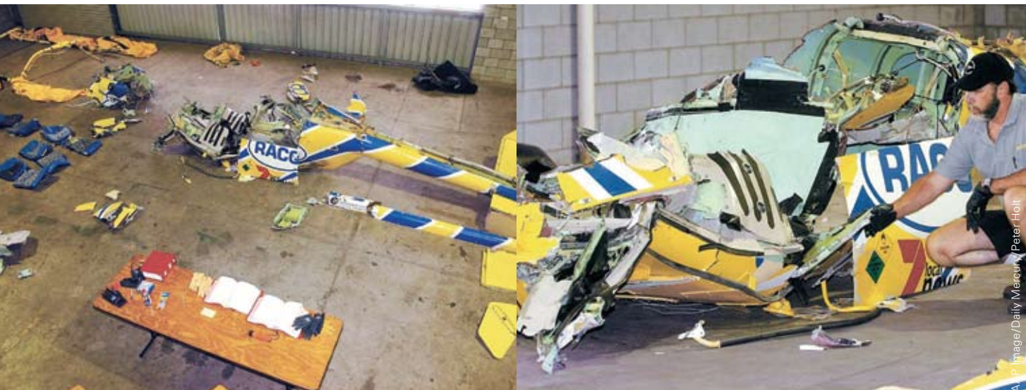
ATSB investigators piece the wreckage together.
