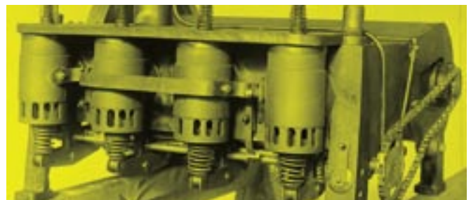
The Flyer engine: The four-cylinder engine had a 4-inch stroke and bore, and produced 12 horsepower at full throttle.
