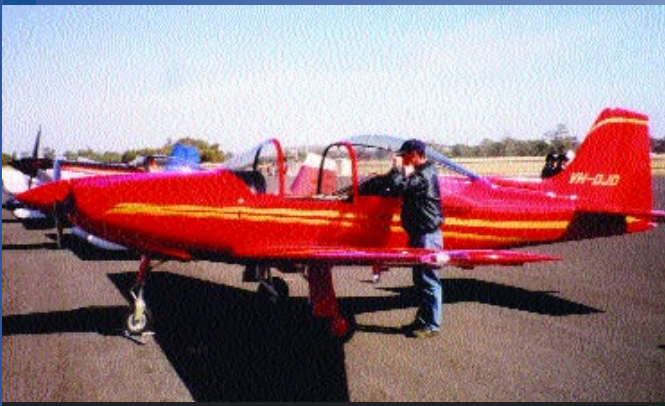
Falco F8L VH-DJD built by the owner, D. Done, NSW. Of wood construction, this aircraft always attracts interest.
