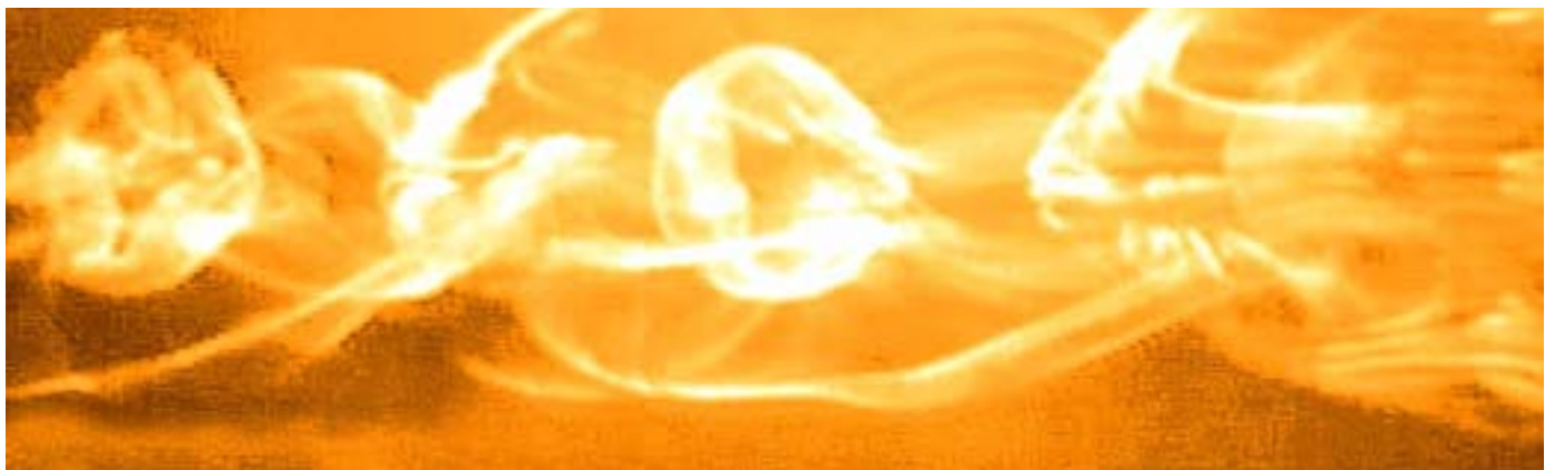
Flow over an oscillating aerofoil. This image was generated in a Monash University experiment on heaving and pitching aerofoils.
