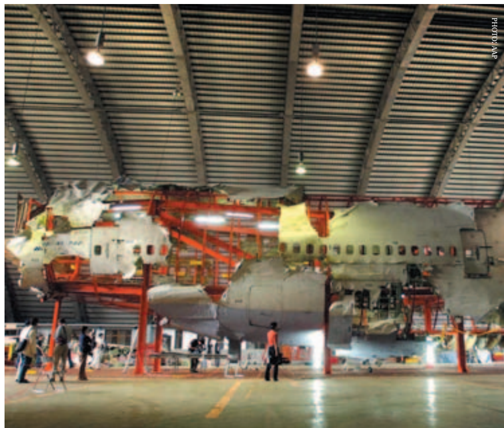
Reconstruction Investigators piece together fragments of Flight 611.
