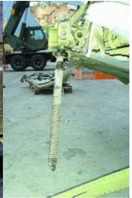
The jackscrew from the horizontal stabiliser of Alaska Airlines flight 261, recovered from main wreckage site.
