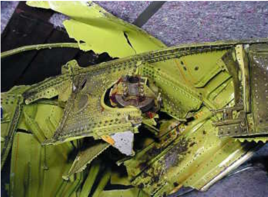
Gimbal nut from Flight 261, shown attached to the front spar of the fin.
